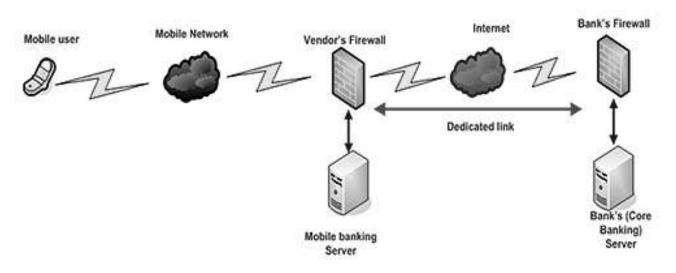
another table for mobile banking users. The customer uses his/her mobile phones to transact through the mobile network. The Mobile banking server in turn talks to the Core banking systems of the bank for user authentication, processing transactions, authorization, etc.
