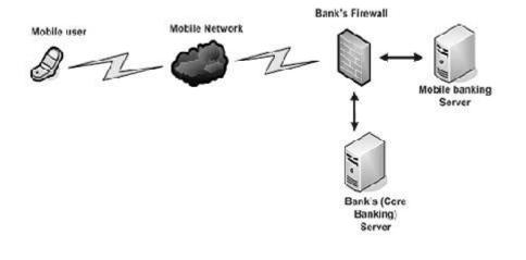
Architecture 1: When the bank provides the service directly to the customer
