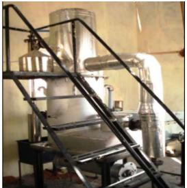
**Figure 1.** 10 kW biomass Gasifier installed at energy park UIT-RGTU Bhopal.
