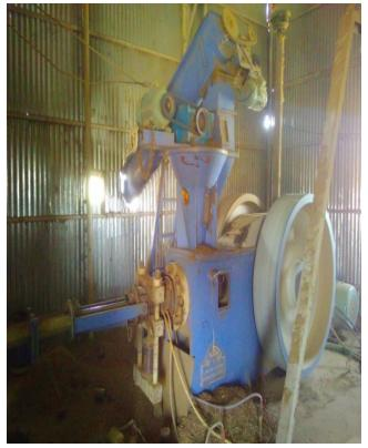
Figure 5. Compresse type Briquetting plant.
