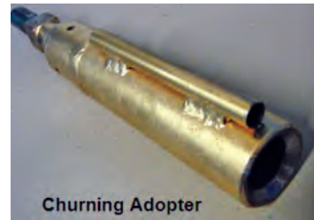
Fig.8 Churning adapter for cable bolts
