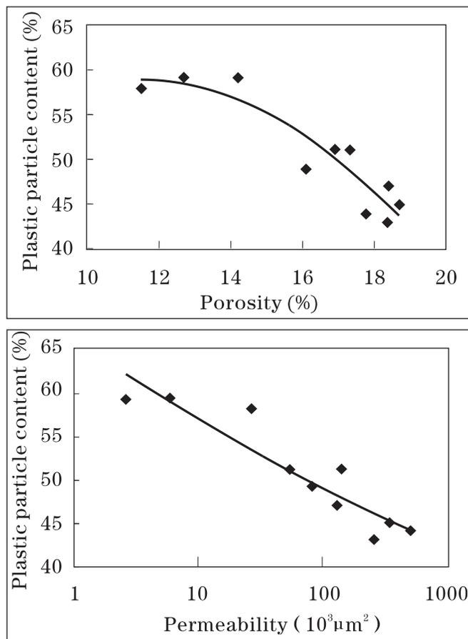
Fig. 1: Quantitative relationship between the content of plastic particle in the reservoir and the porosity and permeability
