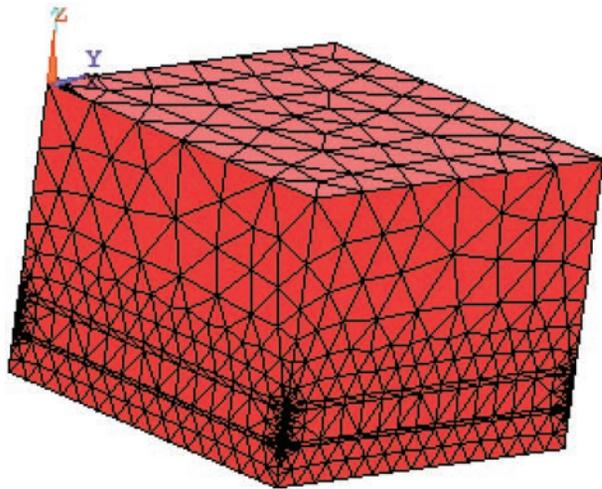
Fig.5 Finite element mesh model of CM panel
