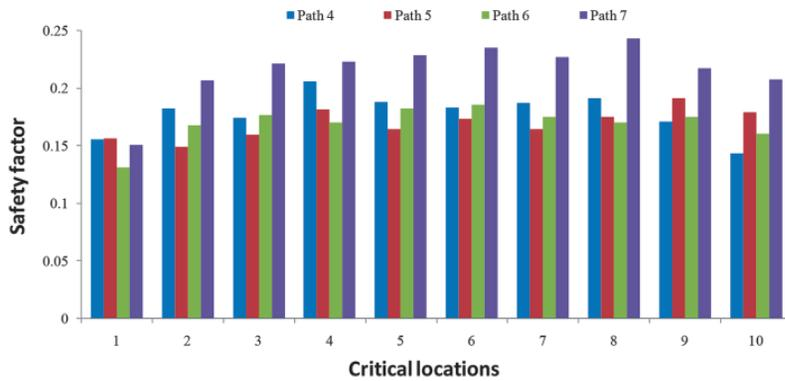
Fig.12 Safety factor of Fender B
