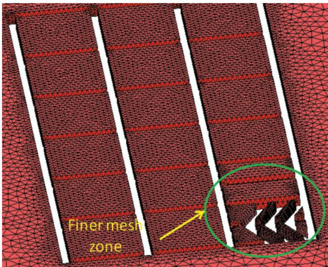
Fig.6 Finite element of coal seam
