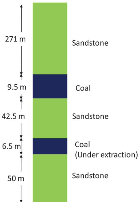
Fig.1 Lithology of mine site used for finite element model
