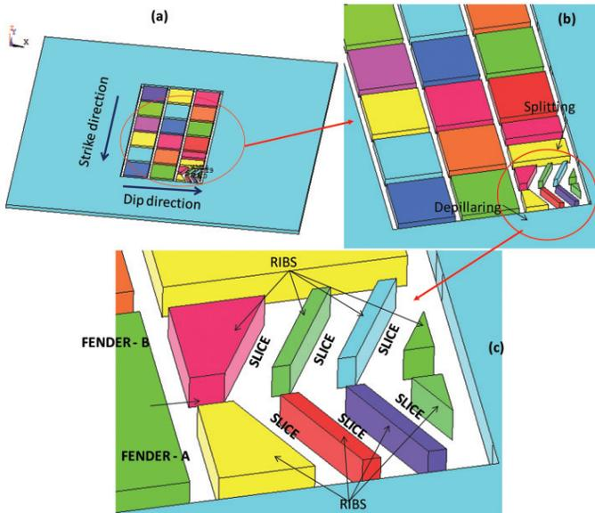
Fig.4 Extraction of the coal seam with continuous miner
