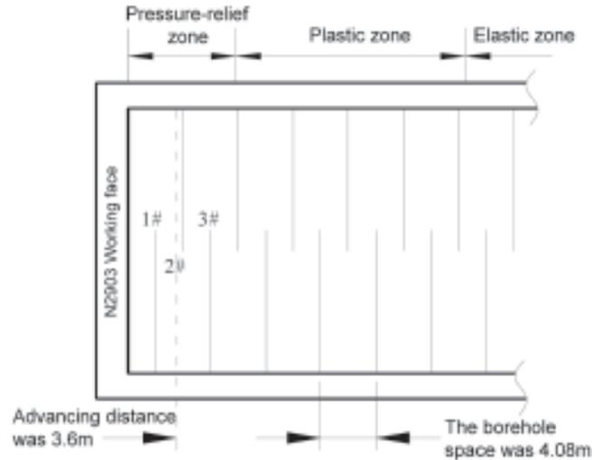
Fig.8 The borehole layout at the mining face
