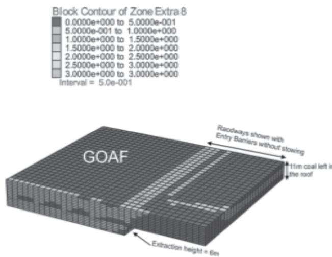
Fig.4 Bottom 6m of coal seam, extracted but very poorly stowed
