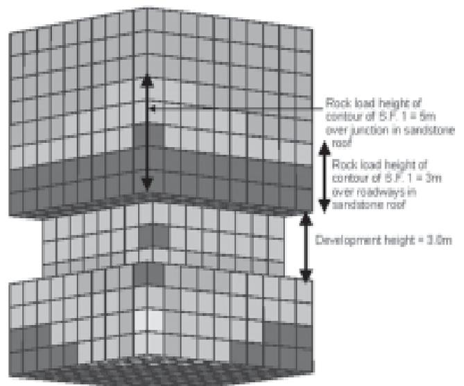
Fig.7 Block contours of safety factor in new development roadways (4m width x 3m height) over stowed lower sections-workings
