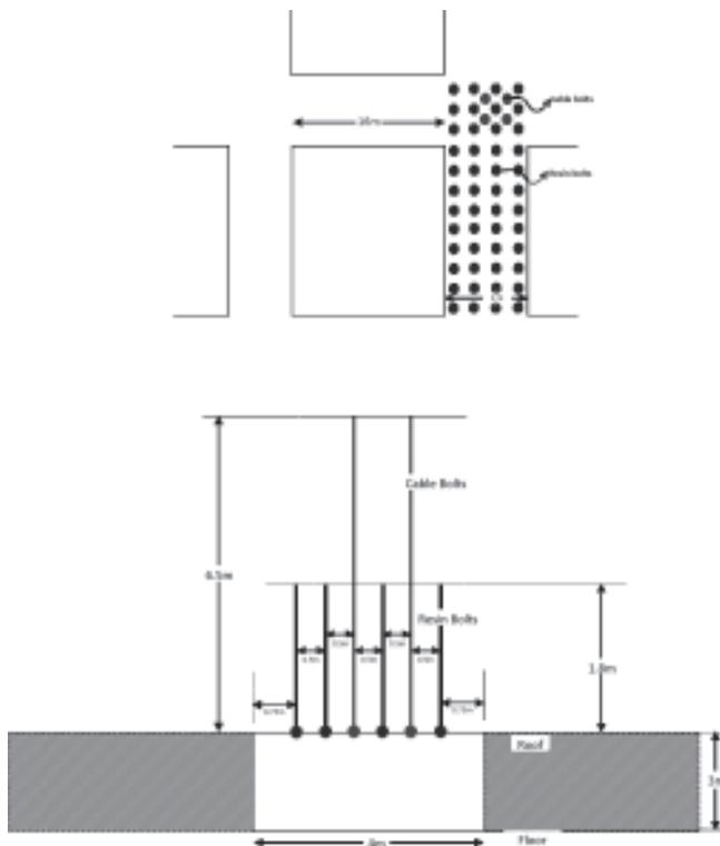
Fig.8 Support design of a roadway 4m (width) with sandstone roof
