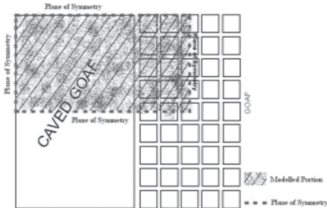
Fig.3 Modelled portion for simulating goaves and existing access and egress galleries (not to the scale) (refer Fig.2)
