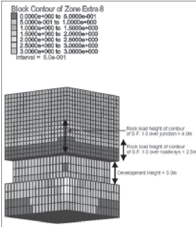
Fig.5 Block contours of safety factor in new development roadways (3.5m width x 3m height) over stowed lower sections-workings
