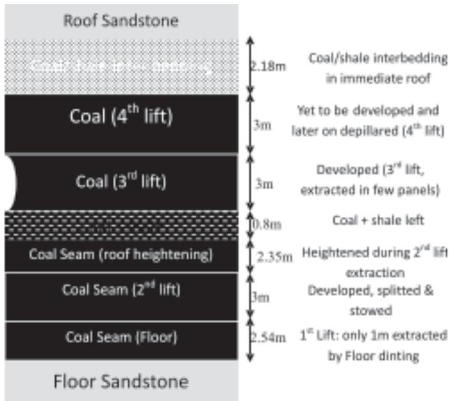
Fig.1 Scheme of extraction methodology followed in Rayatwari seam at CRC mine (not to the scale)
