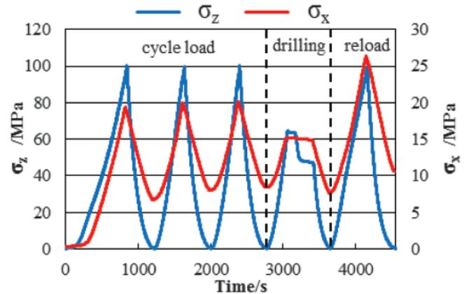
Fig.9 Overall  $\sigma_z$ -time curve and  $\sigma_x$ -time curve
