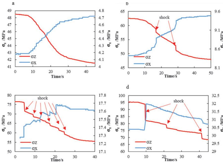
Fig.3 Stress-time curves at an initial  $\sigma_z$  of (a) 50MPa, (b) 65MPa, (c) 80MPa, and (d) 100MPa in the drilling experiment
