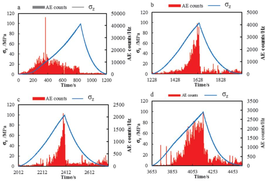
Fig.10  $\sigma_z$ -time curve and AE events in (a) the first, (b) the second, (c) the third, and (d) the last loading and unloading stages, respectively
