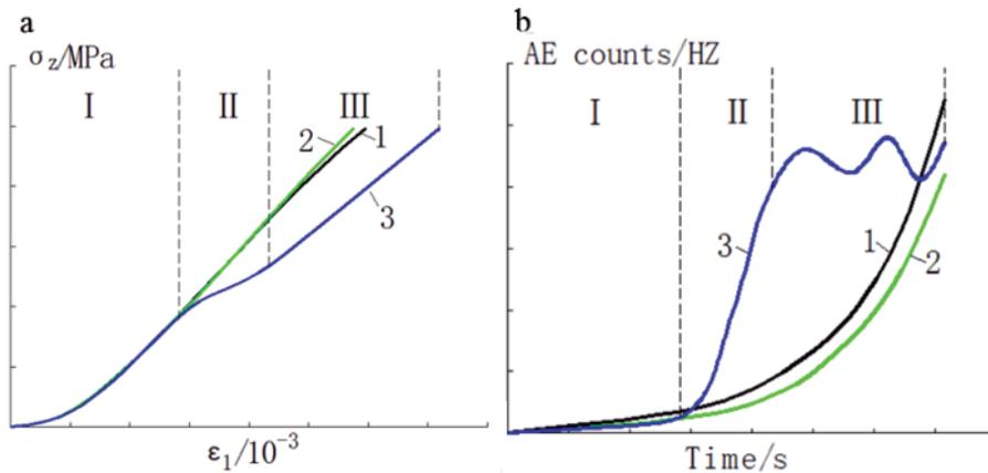
Fig.8 (a)  $\sigma_z$ -strain curves and (b) AE event count-time curves during loading 1, 2, 3-loading curves, reloading of a coal specimen without a hole, reloading curve of a coal specimen with a hole I, II, III -three stages in the reloading curve of a coal specimen with a hole
