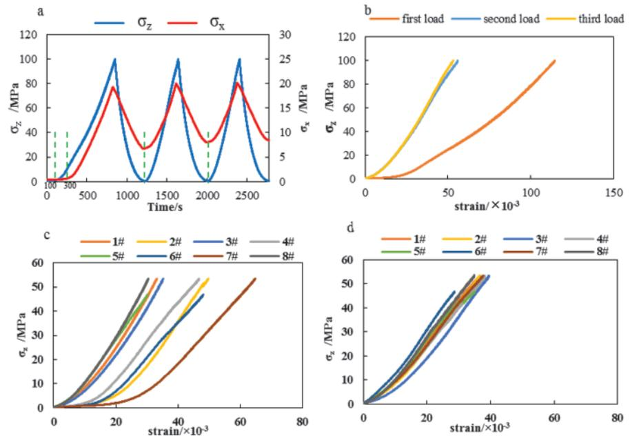
Fig.2 Stress-strain curves and stress-time curves. (a) stress-time curves for cyclic loading and unloading. (b)  $\sigma_z$ -strain curves of the same coal sample under cyclic loading, (c) first loading and (d) second loading  $\sigma_z$ -strain curves for different coal samples, respectively
