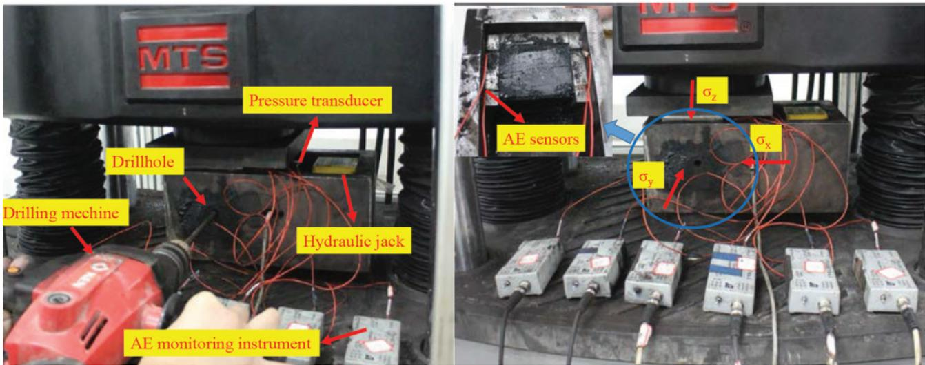
Fig.1 Sketch of the experimental apparatus
