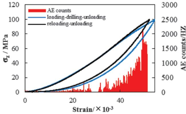
Fig.7  $\sigma_z$ -strain curves during cyclic loading and unloading and AE events during reloading
