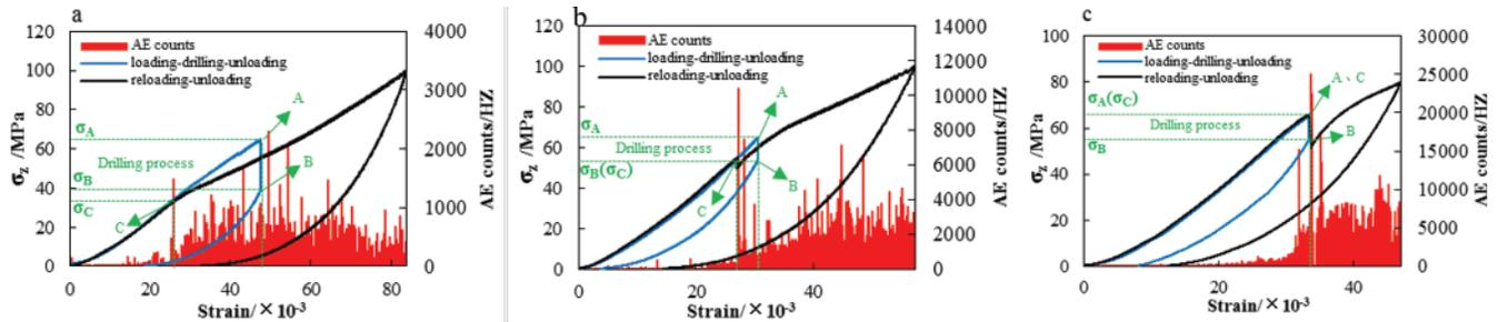
Fig.6  $\sigma_z$ -strain curves and AE events during reloading. The initial vertical stress on the drilled specimen was 65MPa
