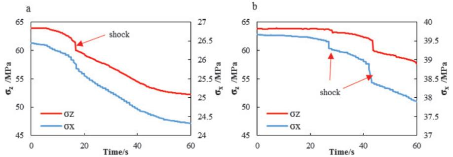
Fig.4 Stress-time curves: (a)  $\sigma_z = 65$ MPa,  $\sigma_x = 26.5$ MPa, and (b)  $\sigma_z = 65$ MPa,  $\sigma_x = 39.5$ MPa
