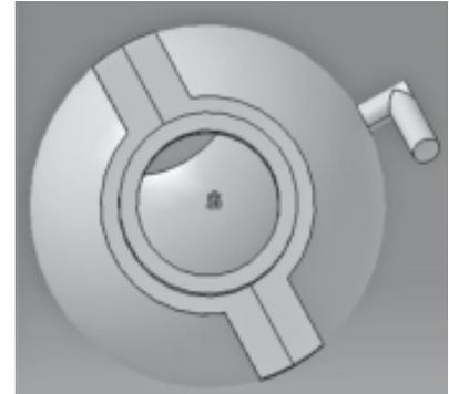
Fig.2 Ball Valve (10° open)
