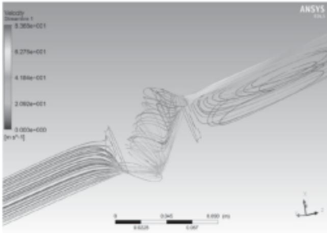
Fig.5 Streamlines of flowing water in the 40° open butterfly valve surface
