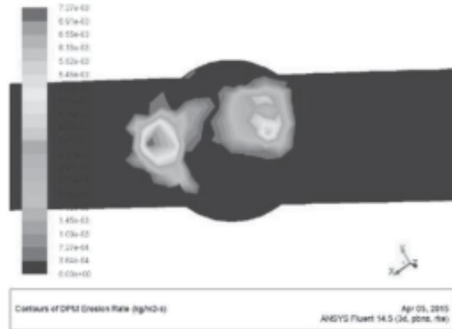
Fig.3 Contour of erosion rate on the 40° open butterfly valve surface
