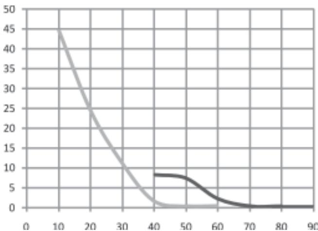
Fig.7 Variation of erosion rate at different valve opening condition for butterfly and ball valve
