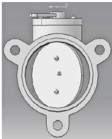
Fig.1 Butterfly valve (40° open)
