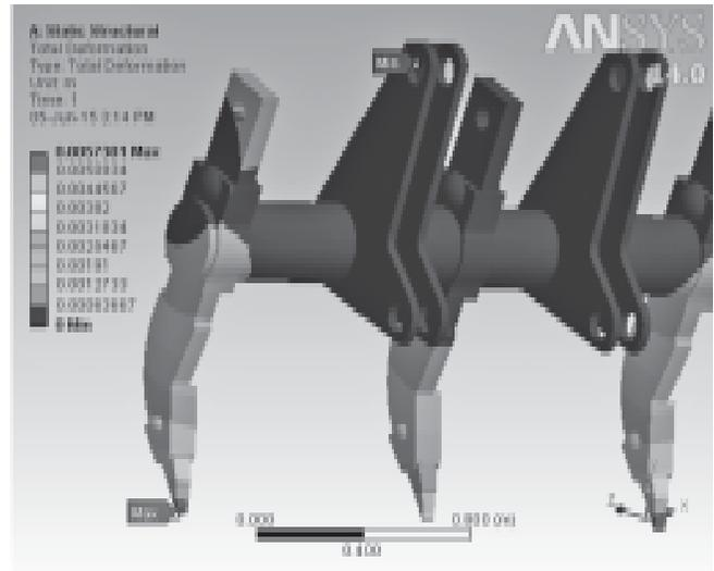
Fig.4(a) Total deformation produced, isometric view 1
