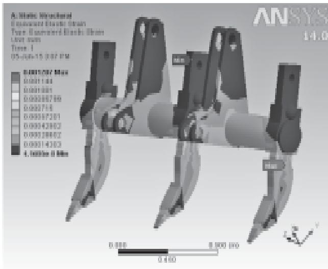
Fig.3(a) Strain induced areas, isometric view 1
