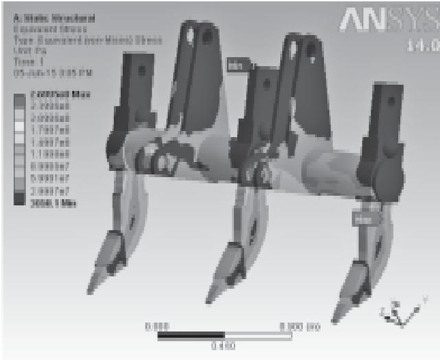
Fig.5(a) Von-mises stress distribution, isometric view 1
