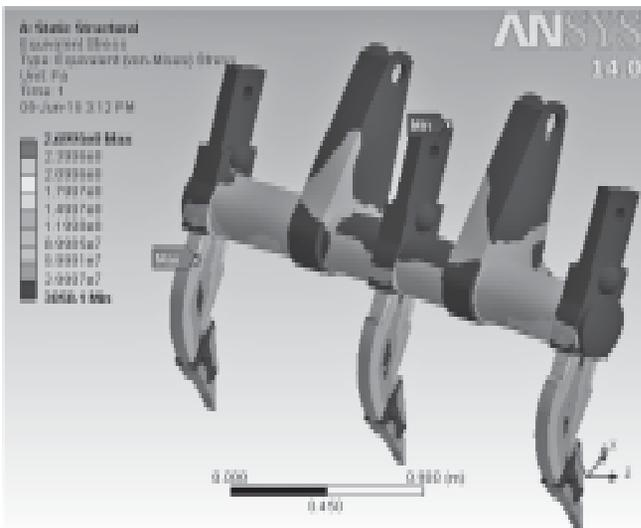
Fig.5(b) Von-mises stress distribution, isometric view 2
