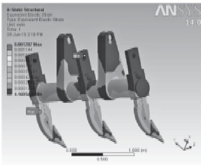
Fig.3(b) Strain induced areas, isometric view 2
