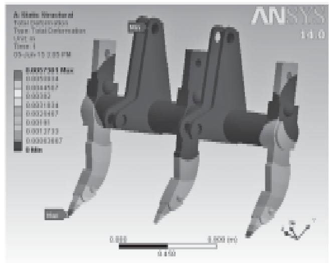
Fig.4(b) Total deformation produced, isometric view 2
