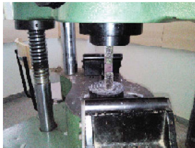
Fig.5: PMCs compression strength testing in UTM
