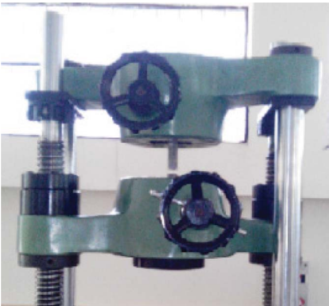
Fig.2: PMCs tensile strength testing in UTM
