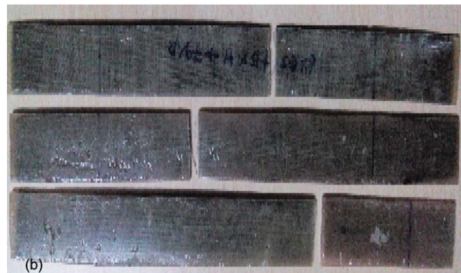
Fig.3(a): PMCs tensile specimens before testing, (b) PMCs Tensile specimens after testing
