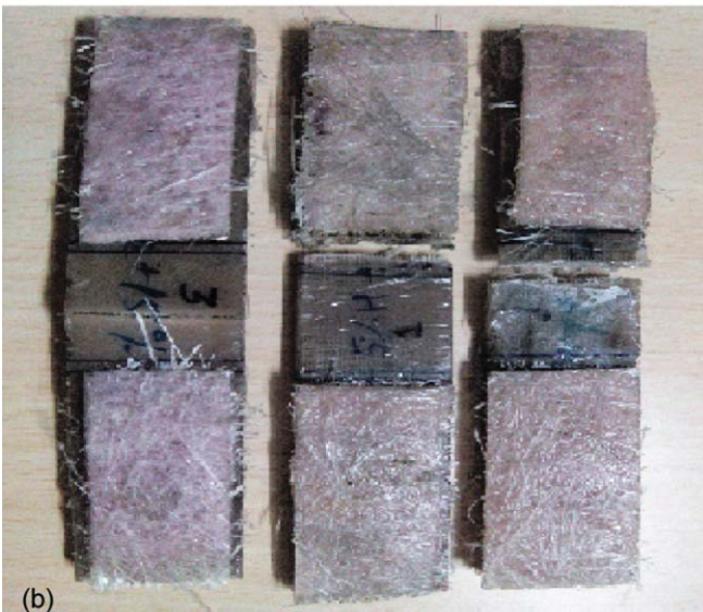
Fig.6(a): PMCs compression specimen before testing, (b) PMCs compression specimens after testing
