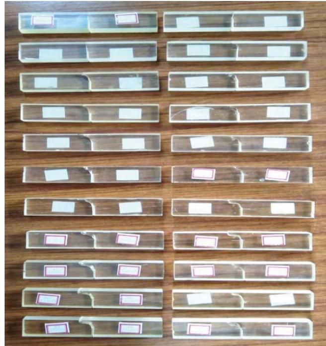
Fig.18: Other fractured ASENb test specimens
