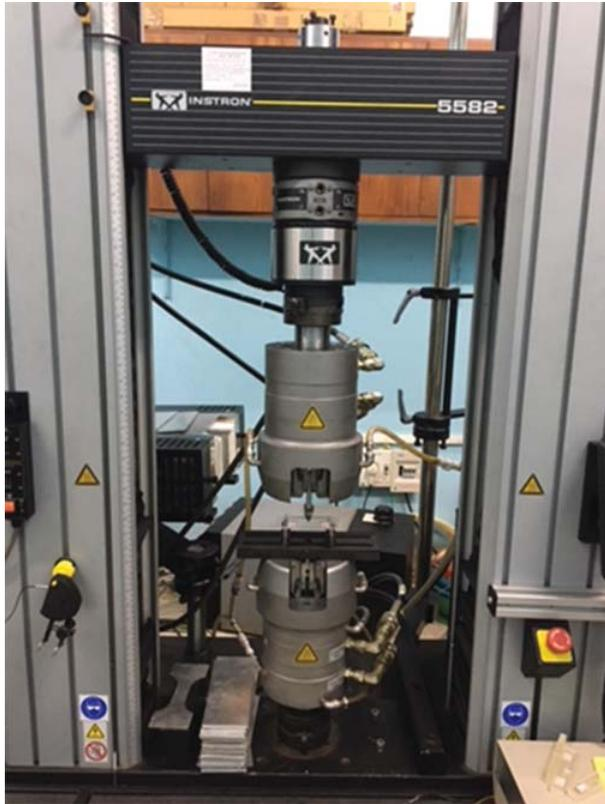
Fig.10: Specimen loaded on Instron 5582 UTM
