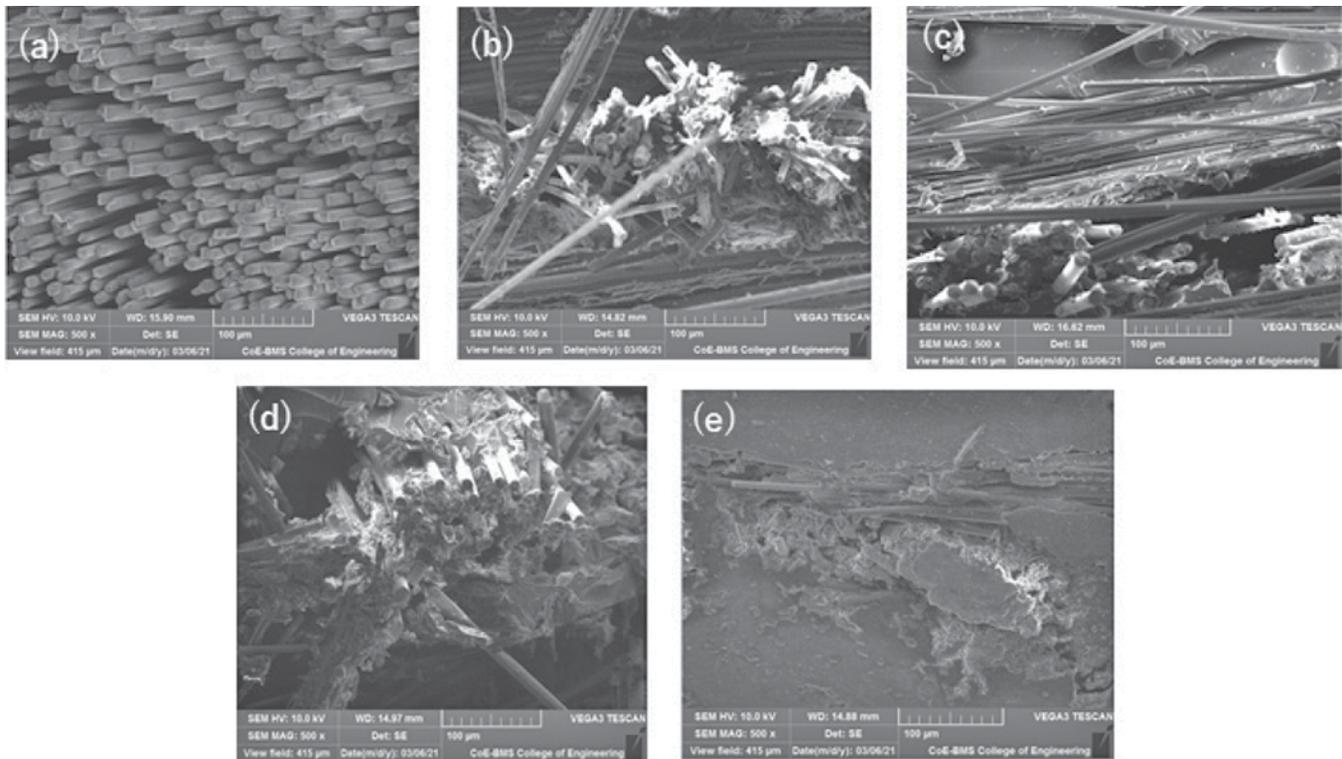
Fig.6: SEM images for (a) L1, (b) L2, (c) L3, (d) L4 and (e) L5 laminates
