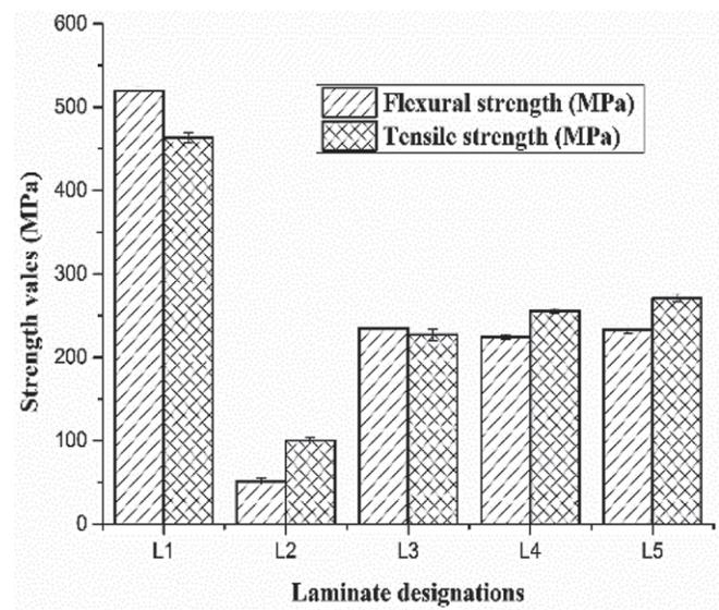
Fig.5: Comparison of tensile and flexural strengths
