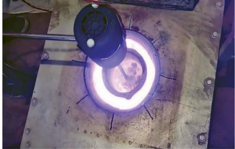
(b) Mixing the reinforcement with base metal
