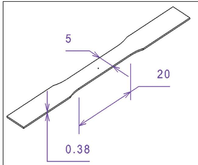
Fig.1. Specification of tensile specimen in mm
