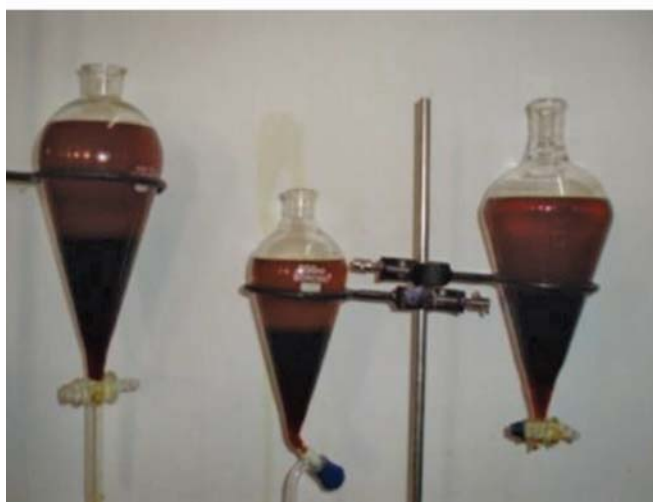
Fig.1: Equipment for conventional transesterification
