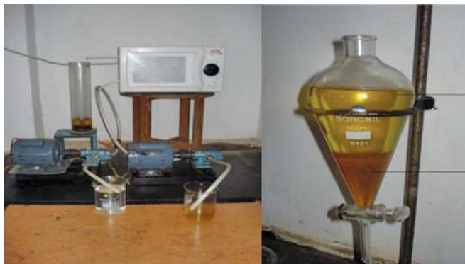
Fig.2: Continuous microwave assisted transesterification method for palm biodiesel preparation
