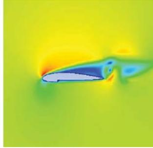
Fig.8: Velocity contours contours at  $0^\circ$  AoA at  $16^\circ$  AoA
