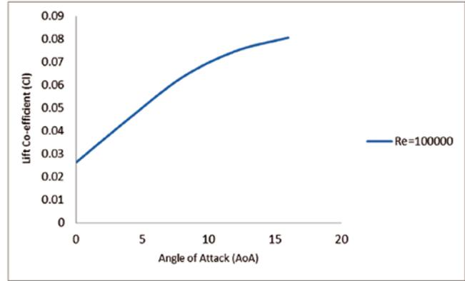
Fig.13: CL vs. AoA graph at 100000 Reynolds number
