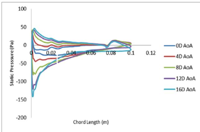
Fig.26: Static pressure vs. chord length graph at varies AoA
