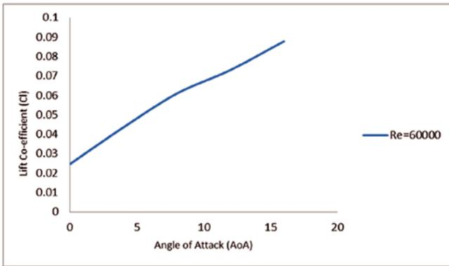
Fig.9: CL vs. AoA graph at 60000 Reynolds number
