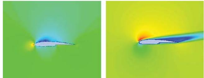
Fig.19. Static pressure contours at 0° AoA
