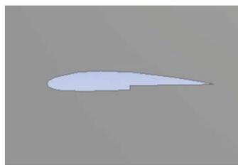
Fig.2: Geometric modelling of airfoil with inward cut at 50% of chord length
