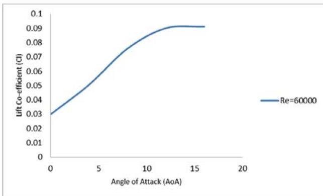
Fig.25: CL vs. AoA graph at 60000 reynolds number
