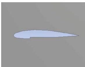
Fig.1: Geometric modelling of airfoil with inward cut at 25% of chord length
