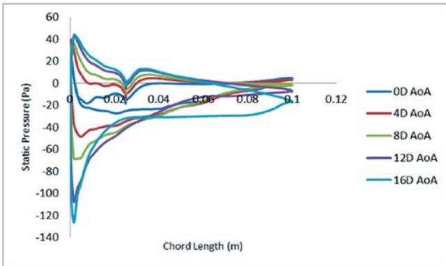
Fig.10: Static pressure vs. chord length graph at varies AoA
