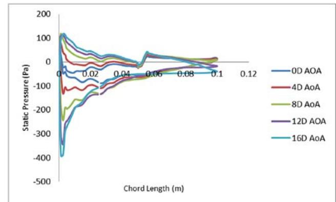
Fig.22: Static pressure vs. Chord length graph at varies AoA
