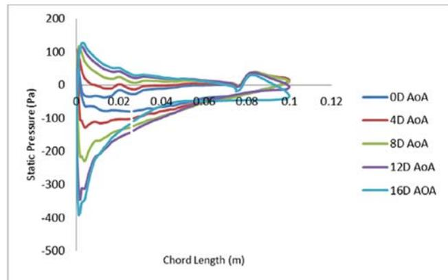
Fig.30: Static pressure vs. chord length graph at varies AoA
