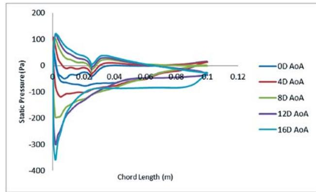
Fig.14: Static pressure vs. chord length graph at varies AoA
