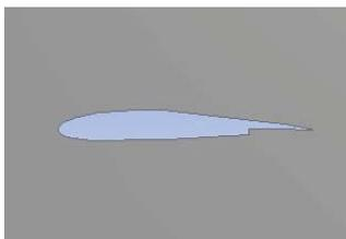
Fig.3: Geometric modelling of airfoil with inward cut at 75% of chord length
