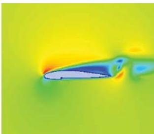
Fig.12: Velocity contours at  $16^\circ$  AoA
