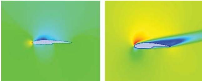
Fig.15: Static pressure contours at 0° AoA
