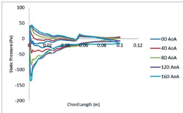
Fig.18. Static pressure vs. chord length graph at varies AoA
