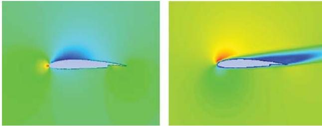
Fig.23: Static pressure contours at 0° AoA
