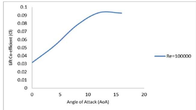
Fig.29: CL vs. AoA graph at 100000 reynolds number
