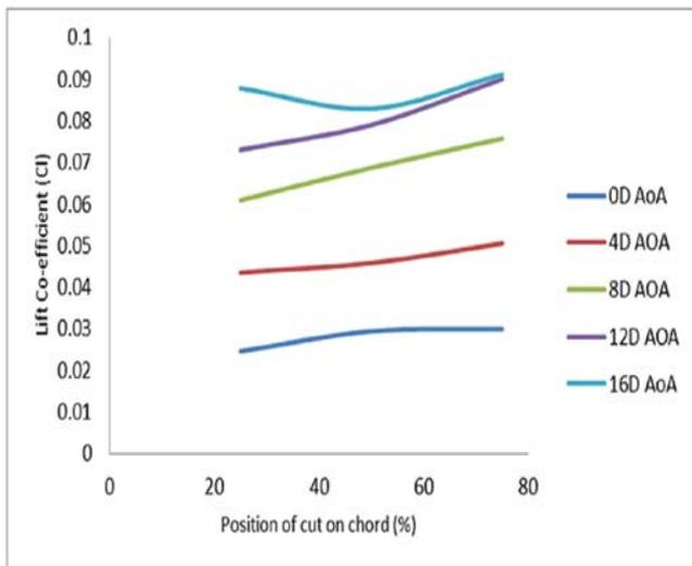
Fig.31: Position of cut on chord vs. lift co-efficient at various AoA
