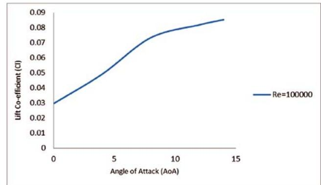
Fig.21: CL vs. AoA graph at 100000 Reynolds number
