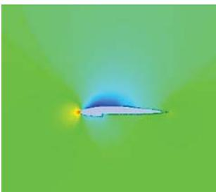
Fig.11: Static pressure contours at  $0^\circ$  AoA
