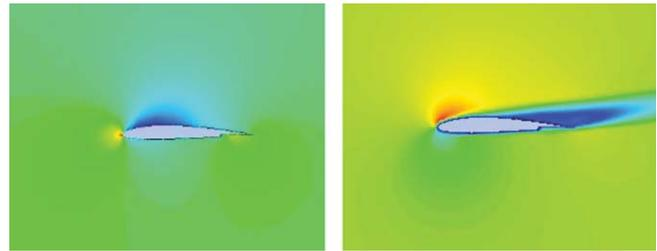
Fig.27: Static pressure contours at 0° AoA
