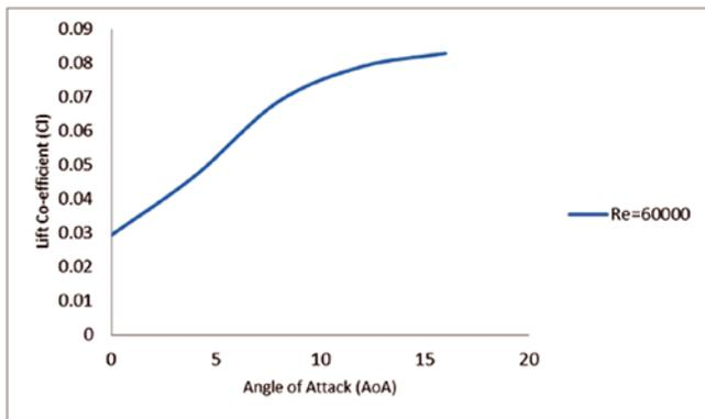
Fig.17. CL vs. AoA graph at 60000 Reynolds number
