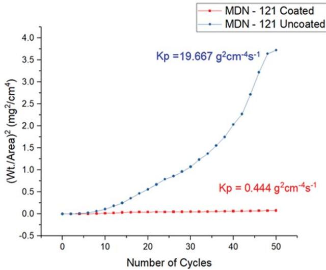
Fig.3: Thermogravimetric data of coated and uncoated MDN-121 subjected to hot oxidation, square of weight gain per unit area versus number of cycles
