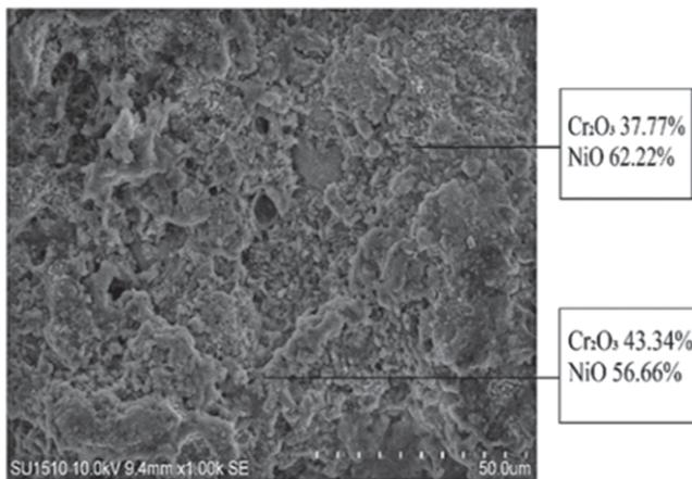
Fig.5: Morphological investigation of MDN-121 uncoated after oxidation
