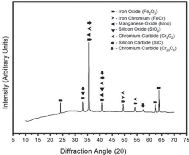
Fig.4: XRD graph of uncoated MDN-121 after oxidation
