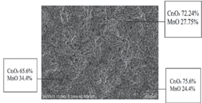
Fig.6: Morphological investigation of MDN-121 coated with  $Cr_3C_2$ -NiCr+NiCrAlY powder after oxidation
