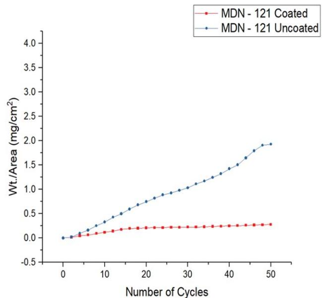
Fig.2: Thermogravimetric data of coated and uncoated MDN-121 subjected to hot oxidation, weight gain per unit area versus number of cycles
