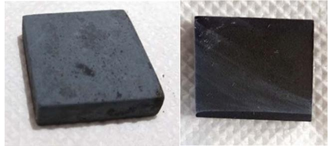
Fig.1: MDN-121 uncoated (left) and coated (right) after oxidation
