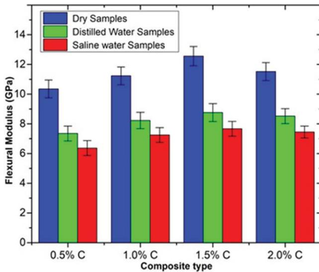
Fig.12: Flexural modulus of cenosphere filled hybrid BGFRECs
