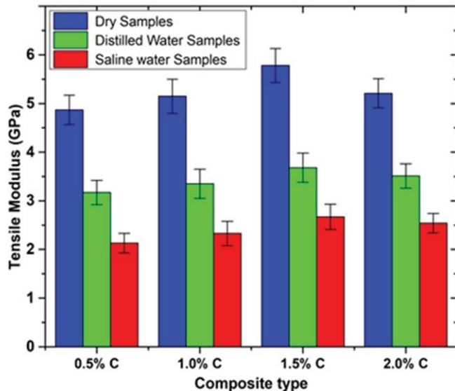
Fig.10: Tensile modulus of cenosphere filled hybrid BGFRECs
