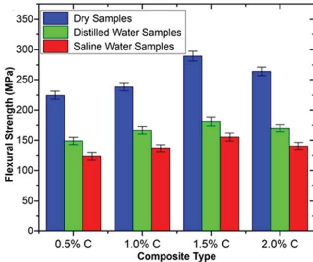
Fig.11: Flexural strength of cenosphere filled hybrid BGFRECs
