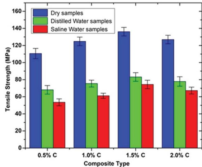
Fig.9: Tensile strength of cenosphere filled hybrid BGFRECs
