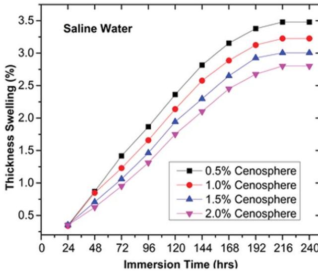
Fig.8: Thickness swelling (%) versus immersion time for saline-water treatment
