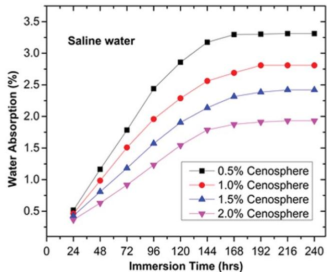
Fig.6: Moisture absorption (%) versus immersion time for saline-water treatment
