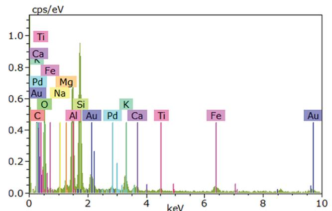
Fig.4 EDX analysis of cenosphere particle
