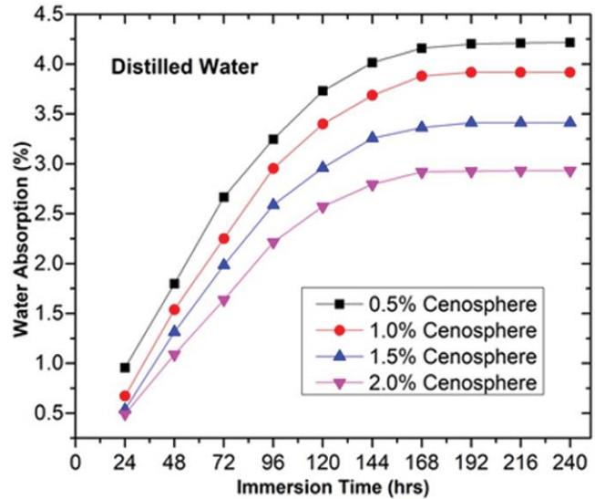
Fig.5: Moisture absorption (%) versus immersion time for distilled-water treatment
