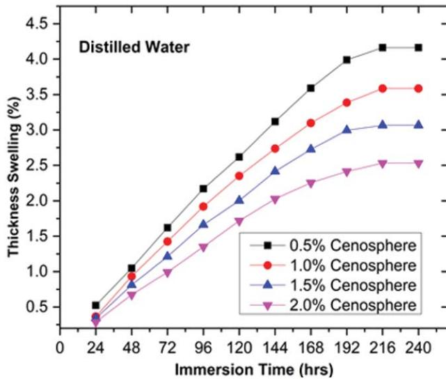
Fig.7: Thickness swelling (%) versus immersion time for distilled-water treatment
