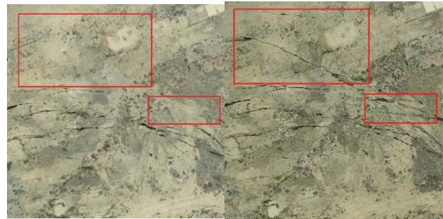
Figure 2. Distribution of surface cracks in 2020 (left) and 2021 (right).
