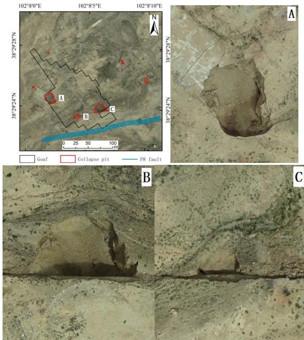
Figure 5. Distribution of surface collapse pits.
