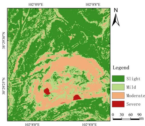
**Figure 7.** Evaluation grade distribution of surface collapse damage degree.
