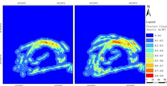
**Figure 4.** Distribution map of surface crack density in 2020 (left) and 2021 (right).
