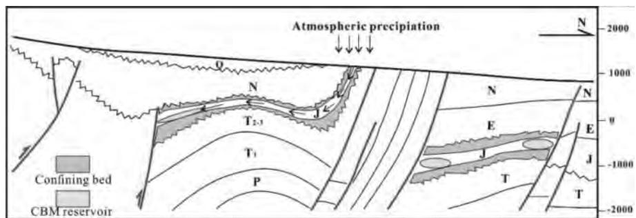
Fig.11 Fault depression enrichment model in the eastern Junggar basin
