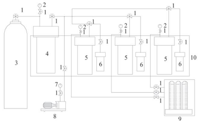
Fig.2 Schematic diagram of gas adsorption and desorption experiment. (1) High-pressure cut-off valve; (2) Accurate pressure meter; (3) High-pressure methane bottle; (4) Gas tank; (5) Big coal sample tank; (6) Small coal sample tank; (7) Vacuum meter; (8) Vacuum pump; (9) Desorption instrument; (10) Thermostatic bath
