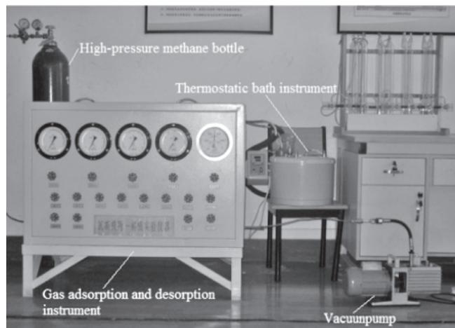
Fig.1 Facility of simulated experiment for gas adsorption and desorption
