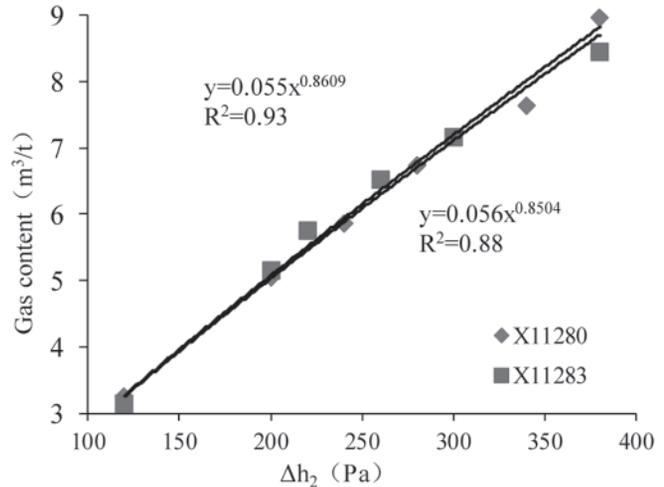
Fig.5 Fitting curves between  $\Delta h_2$  and gas content of different coal samples
