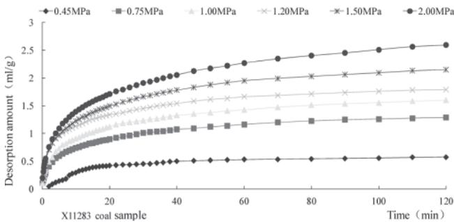
Fig.3 Gas desorption curves of X11283 coal sample under different equilibrium pressure
