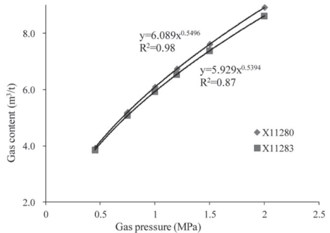
Fig.4 Fitting curves between gas pressure and gas content of different coal samples
