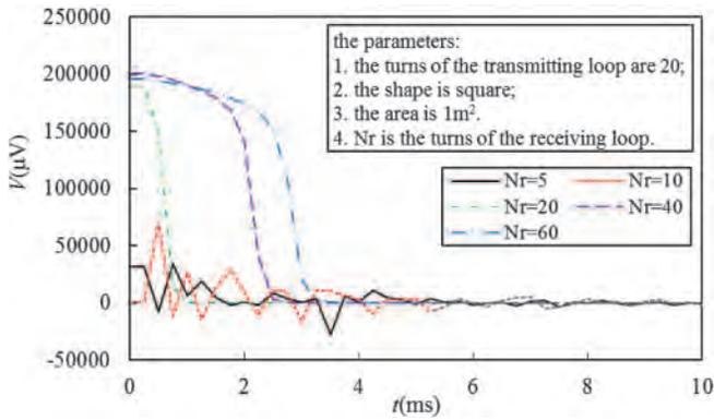
Fig.10 The voltage of received signals versus time at different turns of the receiving loop
