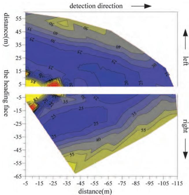
Fig.14 The apparent resistivity contours of the horizontal detection
