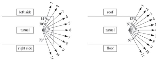
Fig.3 Advanced detection craft of the heading face in underground coal mine
