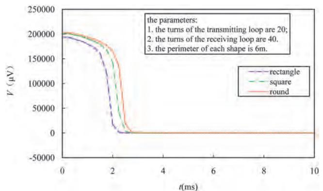
Fig.9 The voltage of received signals versus time at different shapes of the device with overlapping loops
