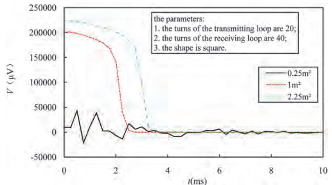
Fig.8 The voltage of received signals versus time at different areas of the device with overlapping loops
