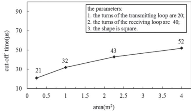
Fig.4 The turn-off time versus the area of the device with overlapping loops
