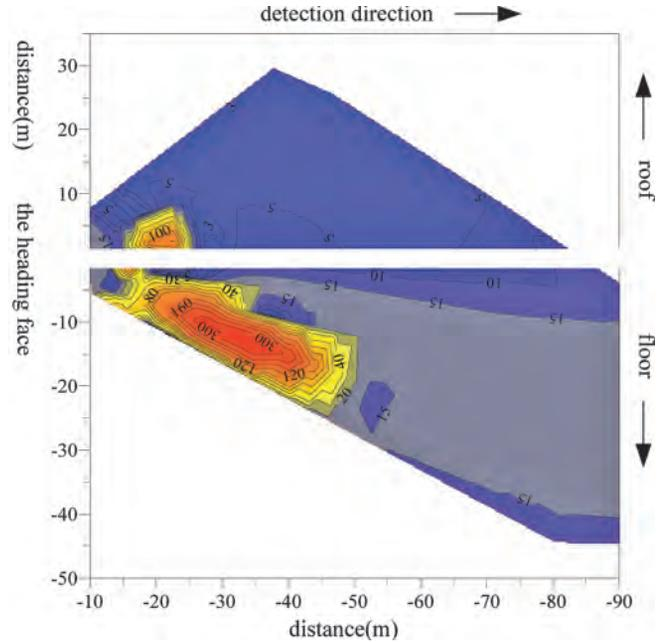
Fig.15 The apparent resistivity contours of the vertical detection
