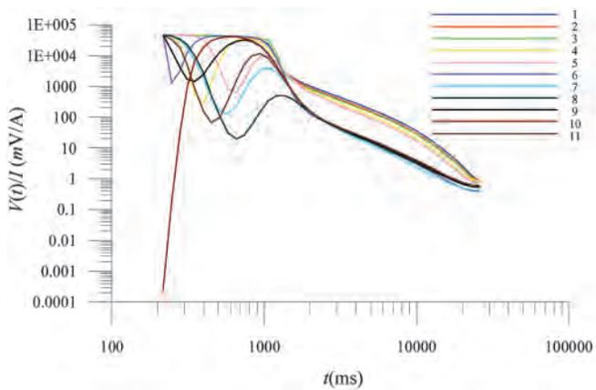
Fig.13 The attenuation curve of the vertical detection:  $V(t)/I$  versus time
