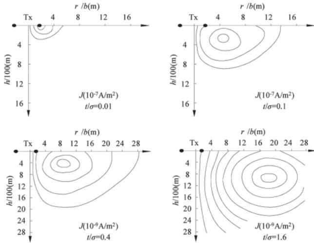
Fig.2 Current density contours in the cross-section via the center of Tx and perpendicular to magnetic lines
