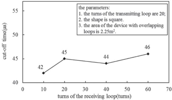
Fig.6 The turn-off time versus the turns of the receiving loop
