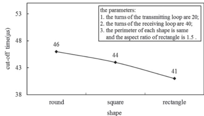
Fig.5 The turn-off time versus the shape of the device with overlapping loops
