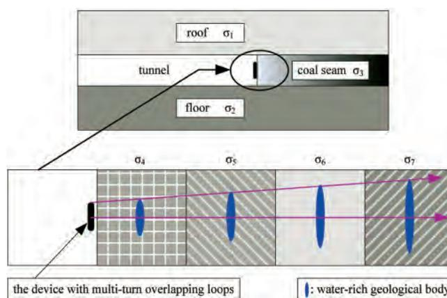
Fig.1 The TEM advanced detection principle
