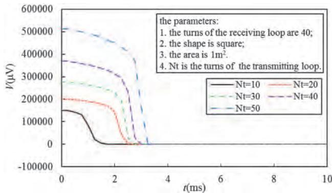
Fig.11 The voltage of received signals versus time at different turns of the transmitting loop
