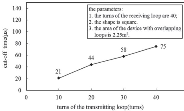
Fig.7 The turn-off time versus the turns of the transmitting loop
