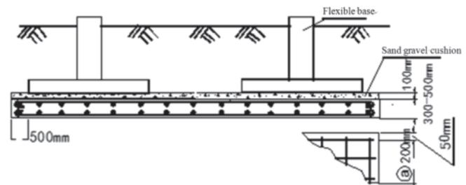
Fig.4 Big slab foundation
