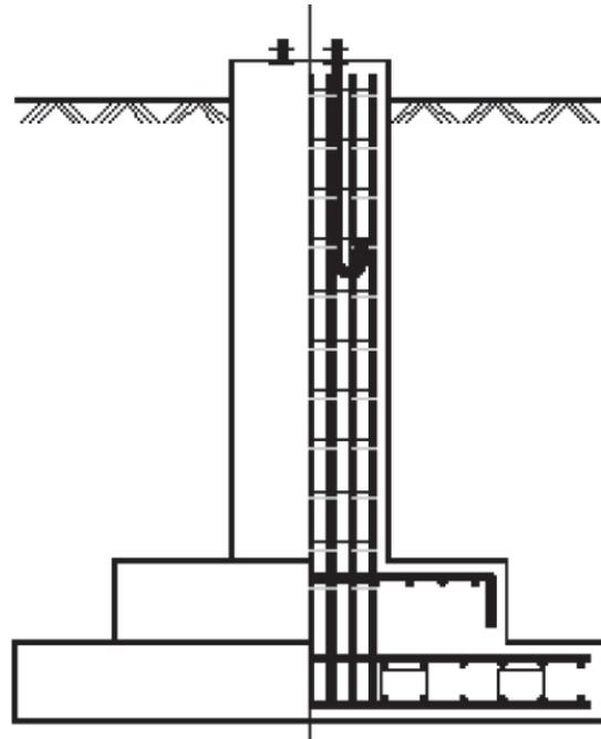
Fig.3 Independent straight column foundation
