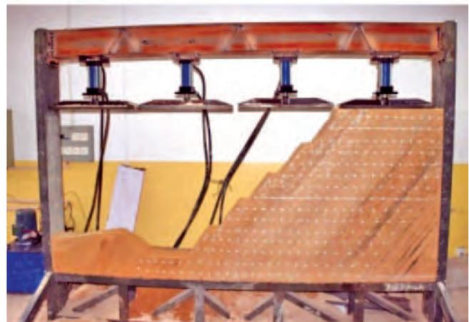
(b) Third loading of model (corresponding to 450 m on-site)
