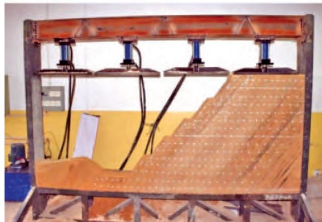
(b) Third loading of model (corresponding to 450 m on-site)
