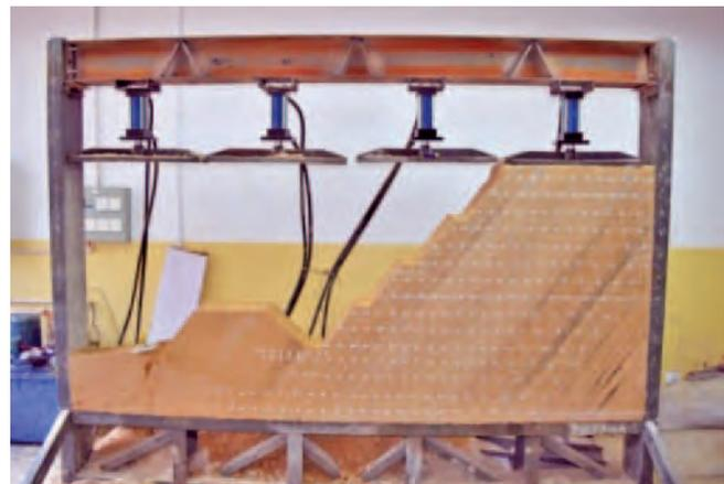
(a) Fourth excavation of model (corresponding to 120 m on-site)
