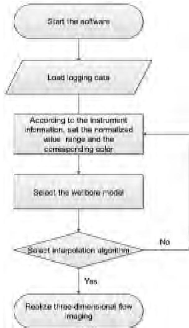
Fig.2 Software design flow chart
