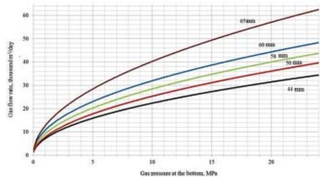
Fig.4 The minimum gas flow rate in a closed inter-ring space, at which the application of technology is acceptable (for various diameters of the central elevator column)
