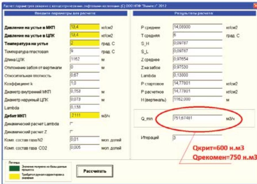
Fig.5 Calculation of the critical rate in the program of LLC NPF Vypmel
