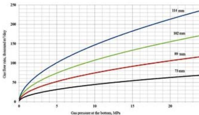
Fig.3 The average daily gas production rate, at the reduction of which it is advisable to use the technology (for various  $D_{head}$  of the main lift column  $D_{mlc}$ )
