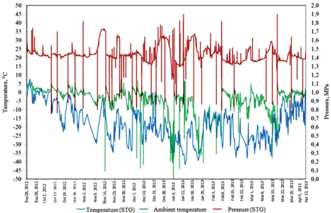
Fig.2 Change in pressure and temperature at the head of the well No. 514 UKPG-5
