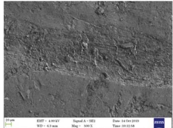
Fig.16 SEM image of the worn surface of the Al LM25 (normal load of 40N, 1.571 m/s sliding velocity at a pin temperature of 90°C)
