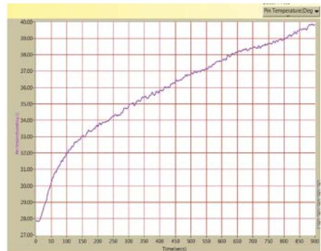
Fig.15 Rise of temperature of the wear pin during dry sliding
