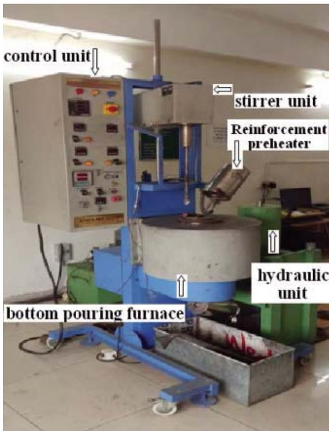
Fig.3 Modified squeeze casting set up
