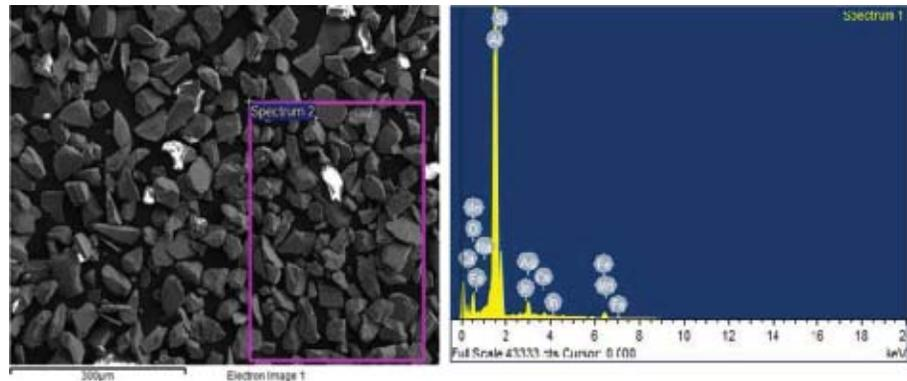
Fig.2 SEM image of steel particles
