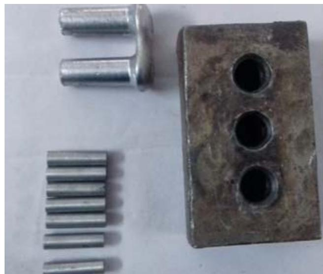
Fig.5 Wear pins with die
