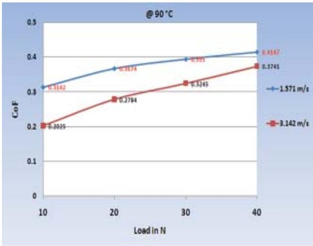
Fig.13 Co-efficient of friction of composites with respect to load, sliding velocity at 90°C
