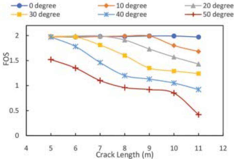
Fig.7 Graphs showing the relation between crack length and crack inclination with FOS
