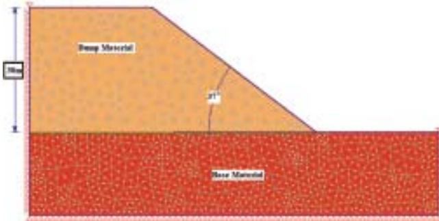
Fig.2 Base model of dump slope with 30m dump height and 37° slope angle
