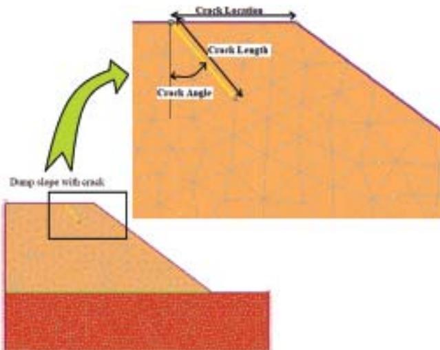
Fig.3 Orientation of crack in the dump slope
