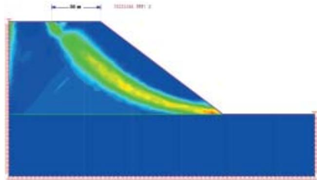
Fig.4 Base dump slope showing the critical failure surface
