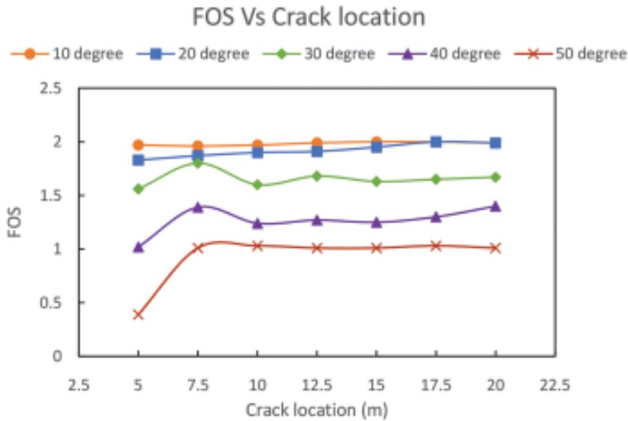
Fig.5 Graph is showing the relation between crack location and crack inclination with FOS
