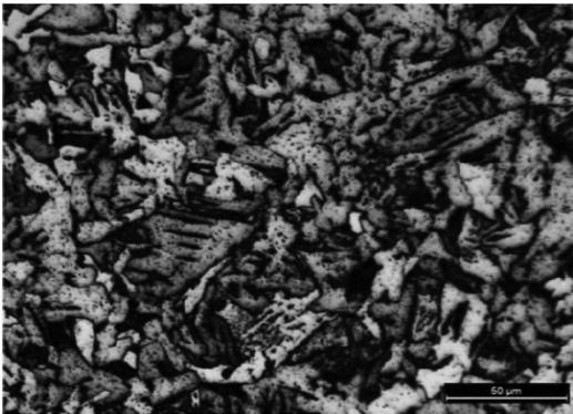
**Fig 7e : FGHAZ (HHI) at a magnification of 500x**
