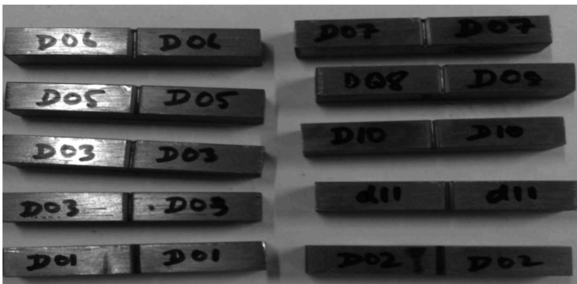
Fig 4 : Standard Charpy specimens of simulated samples
