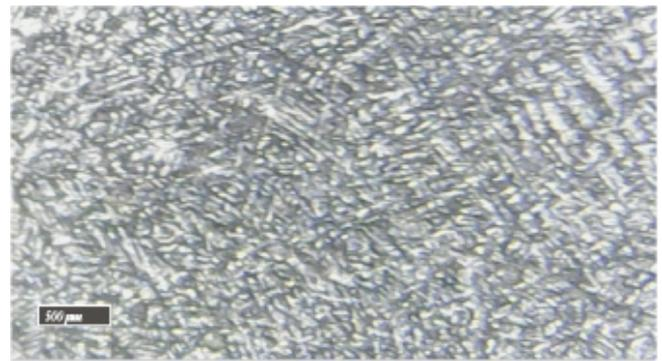
Fig. 4 : Microstructure of solutionized sample
