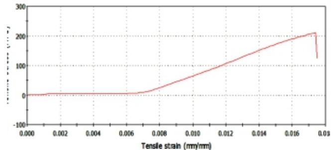
Fig. 3 : Stress-Strain curve for solutionized sample
