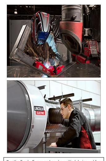
Breathe Freely. Fumes and smoke emitted during welding pose a health hazard. When welding in confined spaces, toxic fumes may accumulate, or shielding gasses may replace breathable air. Use an exhaust hood to remove fumes from the area and ensure enough clean breathing air is available. Some materials specifically require respirators when welding, so consult the manufacturers welding electrode's data sheet, your welding engineer or industrial safety specialist for proper procedures.
