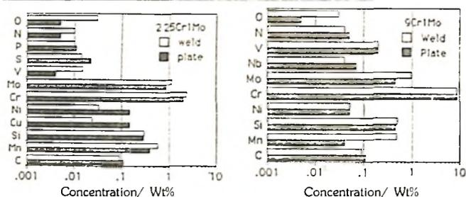
Fig. 1: Comparison of the chemical compositions of weld metal and corresponding wrought steel.
