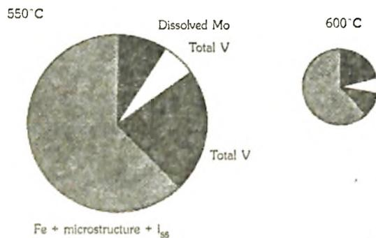
Fig. 5: Factorisation of the  $10^5$ h creep-rupture strength of a  $2\frac{1}{2}$ Cr1Mo steel at the appropriate temperature. The term  $I_{ss}$  represents solid solution strengthening due to elements other than Mo or V. The diameter of each of the pie-charts scales with the creep rupture strength which is 79 and 30 MPa for  $550^\circ\text{C}$  and  $600^\circ\text{C}$  respectively [18].
