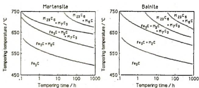
Fig. 2: Measured isothermal transformation diagrams for carbide precipitation reactions in  $2\frac{1}{4}$ Cr1Mo steel. (a) Martensitic starting microstructure; (b) bainitic starting microstructure. Adapted from Baker and Nutting [6].
