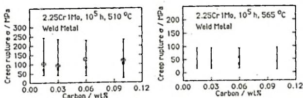
Fig. 7: Calculated (filled circles) with  $\pm 1\sigma$  uncertainties and measured (open circles) stress rupture data for  $2\frac{1}{4}$ Cr1Mo weld metal.
