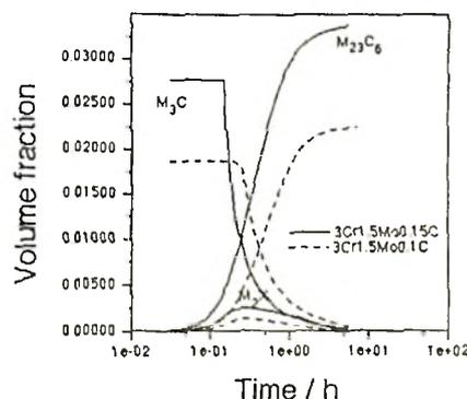
Fig. 4: The calculated evolution of precipitate volume fractions at 600°C for 3Cr1 $\frac{1}{2}$ Mo steel as a function of carbon concentrations and temperature [7,8,17].
