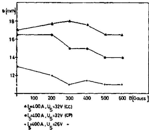
Fig. 1. Effect of magnetic flux density  $B$  on weld width  $b$ .
