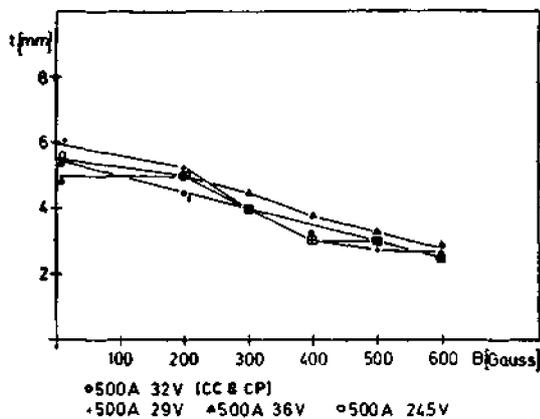
Fig. 5. Effect of magnetic flux density  $B$  on weld penetration  $t$ .
