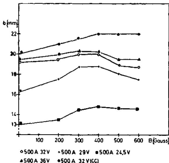
Fig. 2. Effect of magnetic flux density  $B$  on weld width  $b$ .
