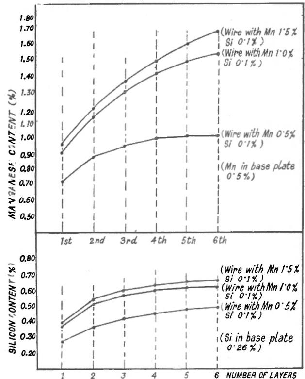
weld deposit, the use of the more expensive higher alloy wire may be dispensed with. If at all higher tensile is required a wire with a small addition of molybdenum may be used.
