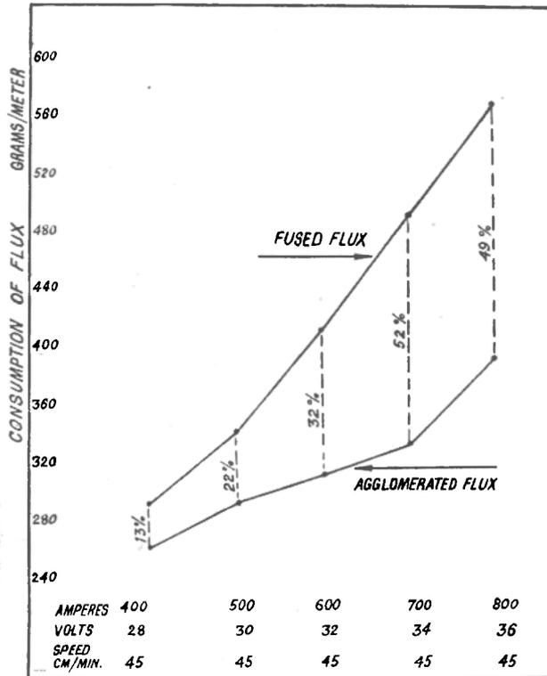
The fear that agglomerated fluxes separate out and consistent results can not be obtained is also not correct. Some German investigators have concluded after extensive research that even in multilayer welds with as many as 75 runs, the weld deposit reveals a very consistent deposit analysis in various layers.
