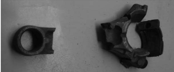
**PLATE 2 FG2 Connecting Rod**
