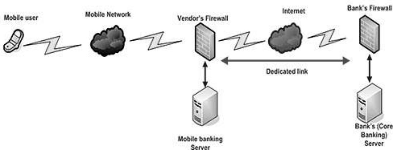
another table for mobile banking users. The customer uses his/her mobile phones to transact through the mobile network. The Mobile banking server in turn talks to the Core banking systems of the bank for user authentication, processing transactions, authorization, etc.
