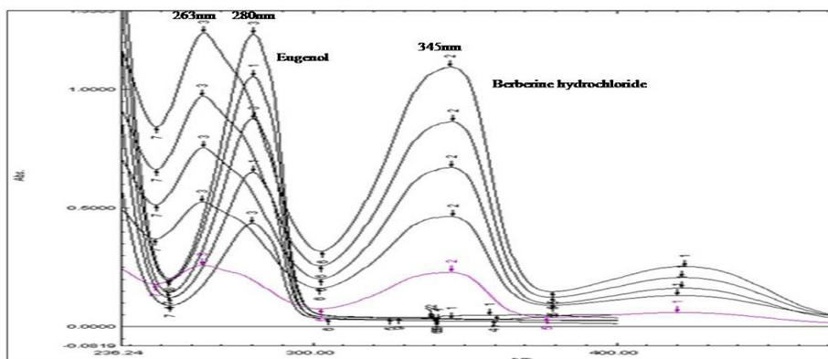
**Figure 1.** Overlain zero-order spectra of the standard solution 4–20  $\mu\text{g/ml}$  of BRB and 2–10  $\mu\text{g/ml}$  of EGN.
