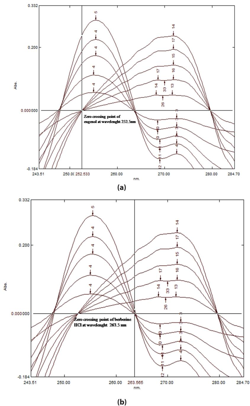
**Figure 2.** (a) First order derivative spectra for the estimation of BRB at 252.5 nm for linearity as EGN is showing zero crossing point. (b) First-order derivative spectra for the estimation of EGN at 263.5 nm for linearity as BRB is showing zero crossing point.
