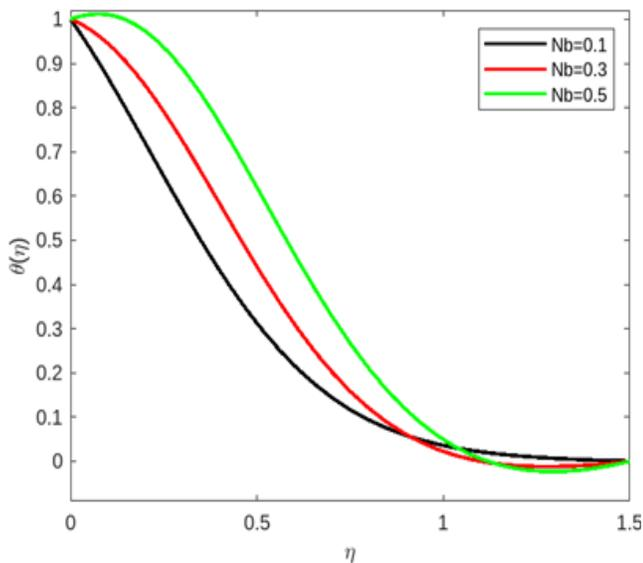
**Figure 2.** Variations in temperature profile  $\theta(\eta)$  with Brownian motion ( $Nb$ ).
