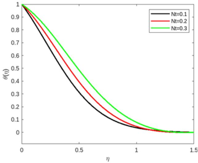
**Figure 1.** Variations in temperature profile  $\theta(\eta)$  with thermophoresis parameter ( $Nt$ ).
