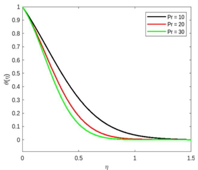
**Figure 4.** Variations in temperature profile  $\theta(\eta)$  with Prandtl number ( $Pr$ ).
