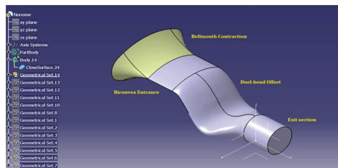
Figure 4: Geometry of the Serpentine Inlet Model
