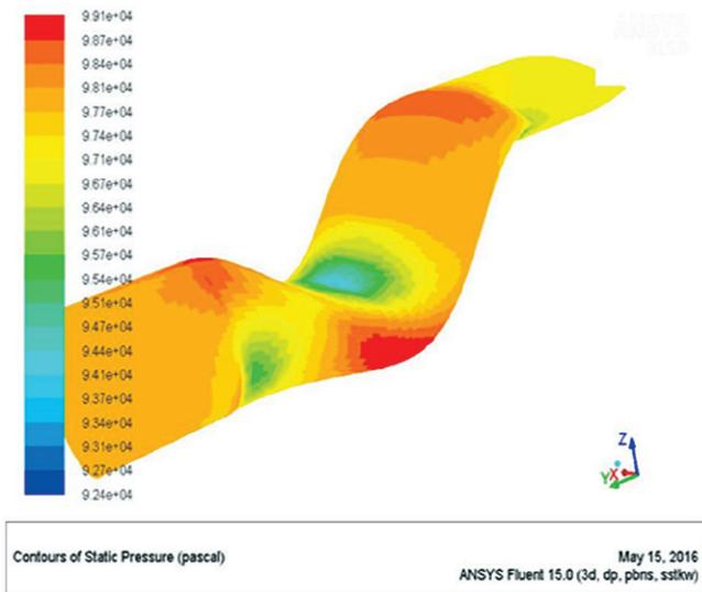
Figure 11: Static pressure contours for baseline ducts
