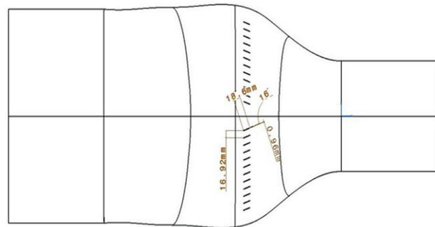
**Figure 5: Vortex generator specifications**
