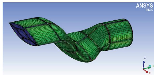
**Figure 6: Discretization of serpentine duct baseline geometry**
