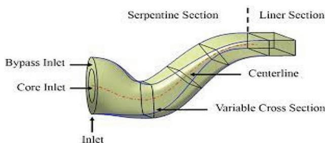
Figure 1: Representation of S-Duct
