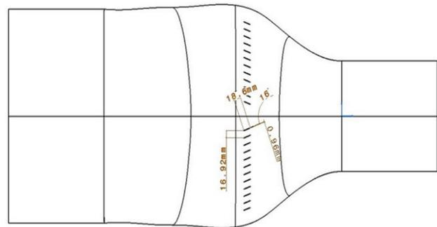
**Figure 5: Vortex generator specifications**
