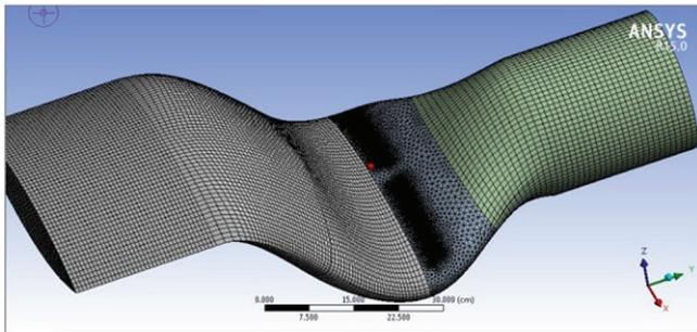
**Figure 7:** Discretized serpentine duct with Vortex generator
