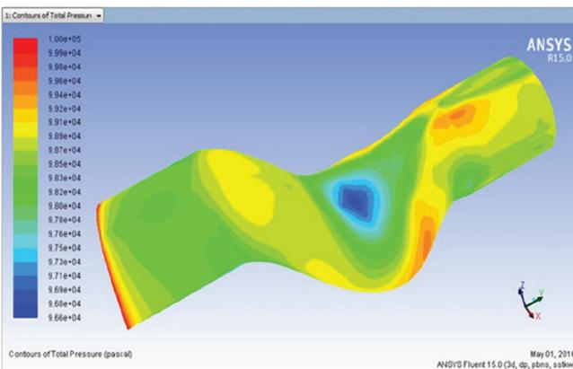
Figure 12: Total pressure contour for baseline duct
