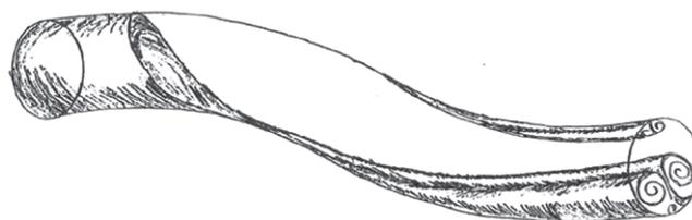
Figure 2: Serpentine duct with natural vortices
