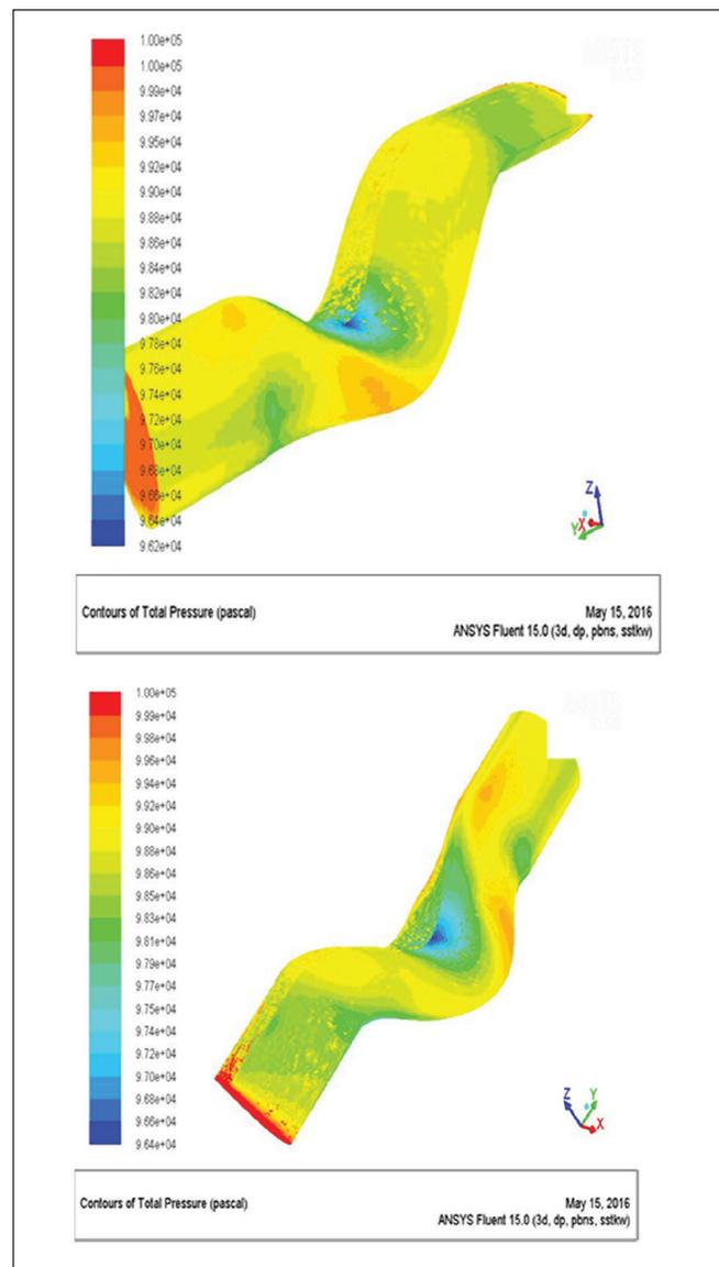
**Figure 8:** Total Pressure contours for baseline ducts
