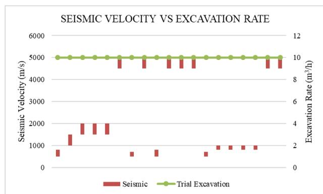
Figure 14. The relationship between seismic velocity and excavation rate at Kota Tinggi site.
