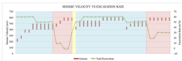
Figure 8. The relationship between seismic velocity and excavation rate at Nilai site.
