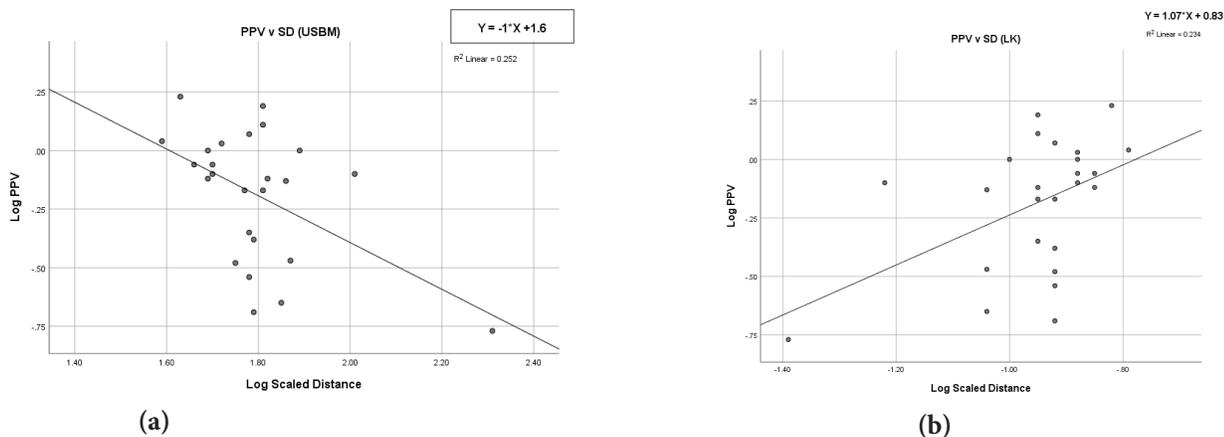
**Figure 4.** Regression SPSS Analysis for log (PPV) against log (Scaled Distance) using equations from (a) USBM and (b) Langefors-Kihlstrom, (1963).
