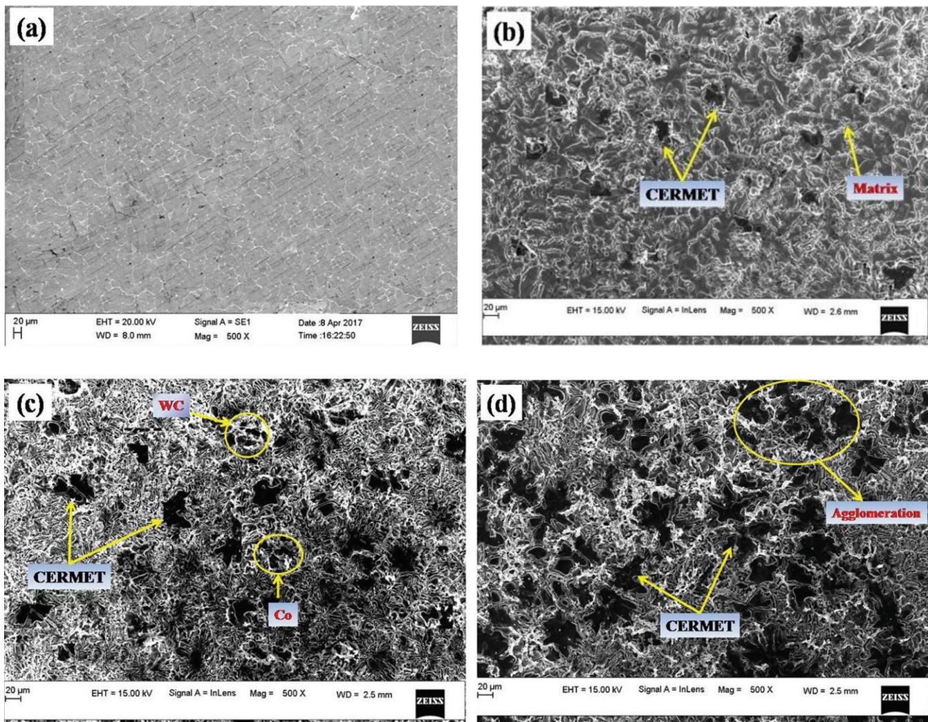
**Figure 3** (a-d): SEM images of (a) As cast 7075Al, (b) 7075Al + 6wt.% Composite, (c) 7075Al + 9wt.% Composite and (d) 7075Al + 12wt.% Composite
