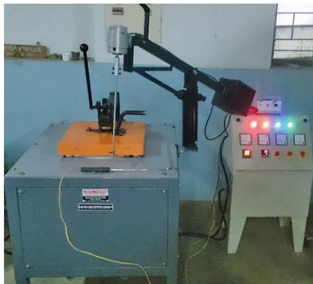
Figure 1: Apparatus used in preparation of composite [Stir casting setup]
