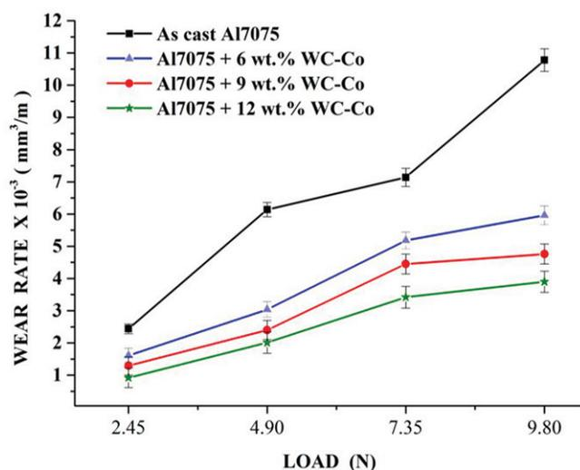
**Figure 7:** Wear rate of (a) as cast 7075Al and 7075Al reinforced with WC-Co particulate composite with different loads at constant sliding speed and sliding distance
