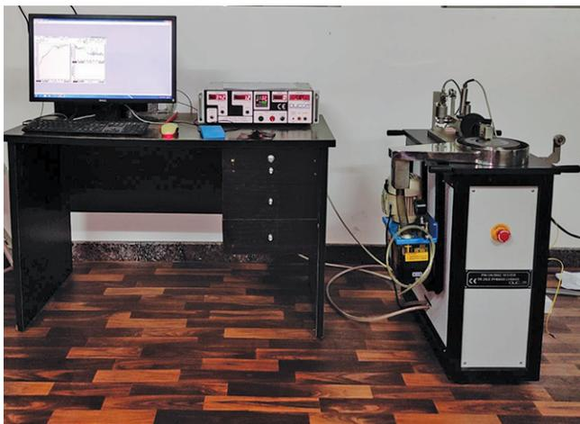
**Figure 2:** Apparatus used in testing the composite wear resistance
