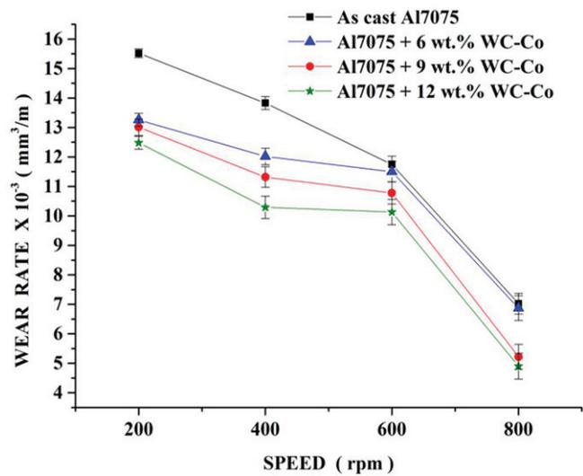
Figure 6: Wear rate of (a) as cast 7075Al and 7075Al reinforced with WC-Co particulate composite with different speed at constant load and sliding distance
