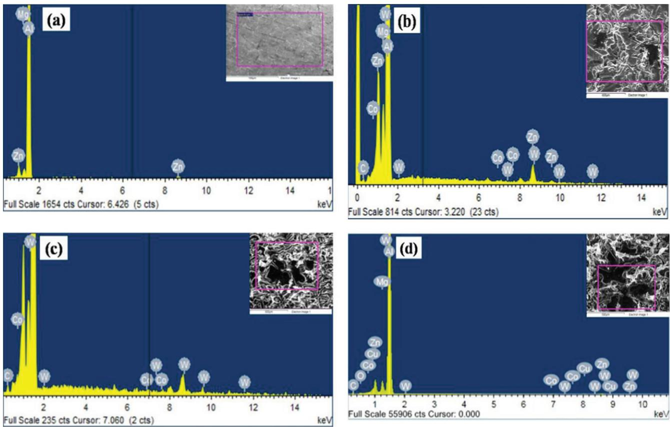
Figure 4 (a-d): EDAX analysis of (a) As cast 7075Al, (b) 7075Al + 6wt.% Composite, (c) 7075Al + 9wt.% Composite and (d) 7075Al + 12wt.% Composite
