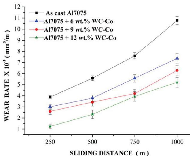
**Figure 8:** Wear rate of (a) as cast 7075Al and 7075Al reinforced with WC-Co particulate composite by varying sliding distance at constant sliding speed and load
