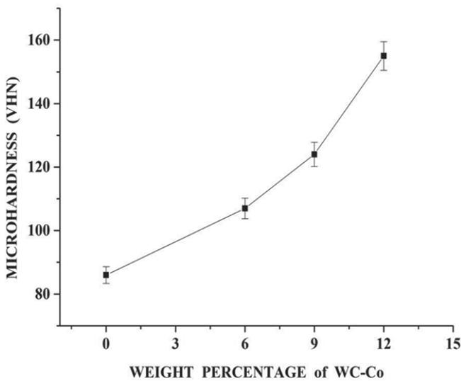
Figure 5: Micro hardness of as cast 7075Al and 7075Al reinforced with 6, 9, 12 wt.% WC+Co composite
