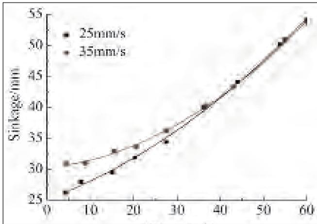
(a) The variation of sinkage with slip ratio
