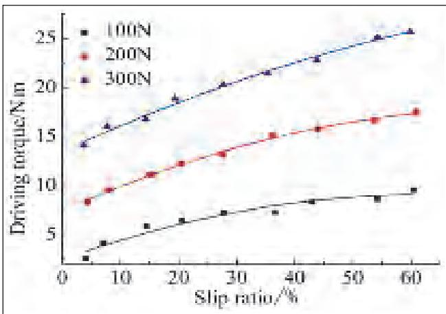
(c) The variation of driving torque with slip ratio
