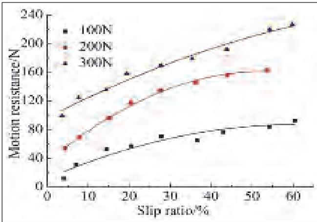
(d) The variable of motion resistance with slip ratio
