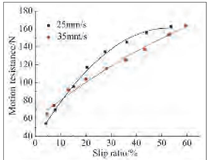
(d) The variable of motion resistance with slip ratio
