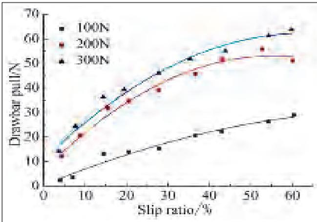
(b) The variable of drawbar pull with slip ratio
