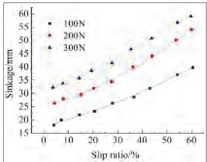
(a) The variation of singkage with slip ratio
