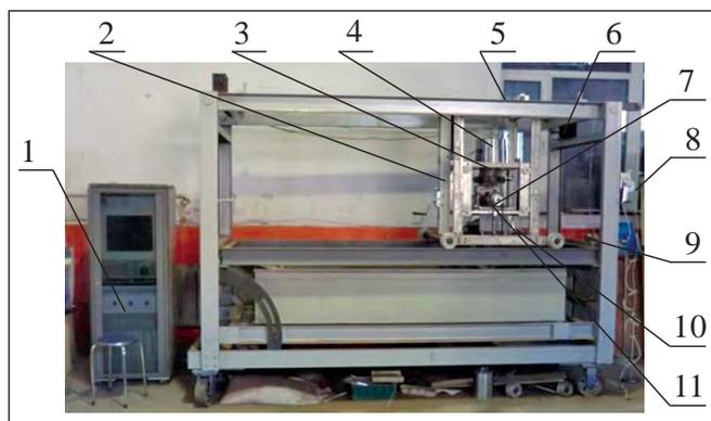
Fig. 1. Lunar soil-wheel test bin
