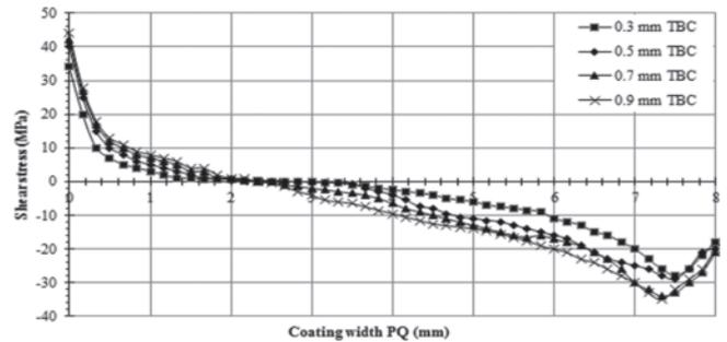
Fig.10 Shear stress variation as a function of coating thickness for substrate surface
