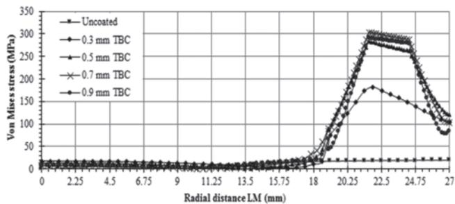
Fig.6 Normal stress variation as a function of coating thickness for top surface
