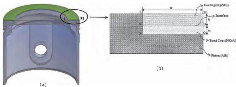
Fig.1(a) Half part of partially coated piston, and (b) Parameters used during analysis
