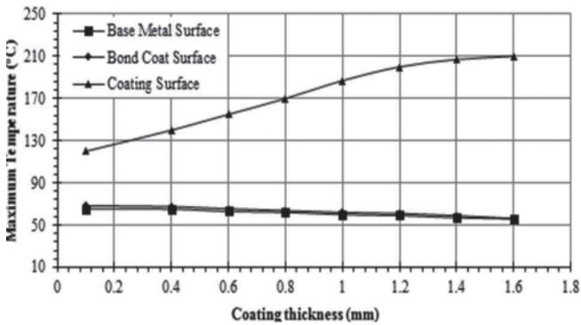
Fig.5 Maximum temperature variation as a function of coating thickness
