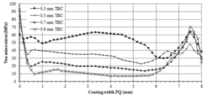
Fig.9 Normal stress variation as a function of coating thickness for substrate surface
