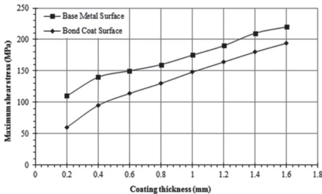
Fig.12 Maximum shear stress variation with coating thickness for interfaces
