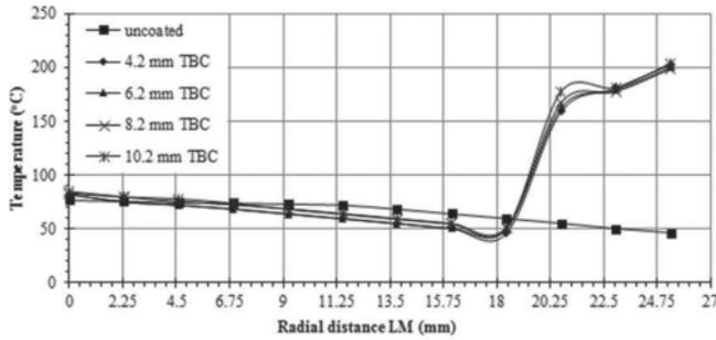
Fig.4(b) Top surface temperature distribution with coating width
