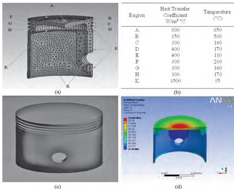
Fig.2(a) Boundary Conditions of the Piston [10] (b) Heat transfer coefficient and temperature values for different regions (c) Model used for analysis, and (d) Temperature distribution for uncoated piston
