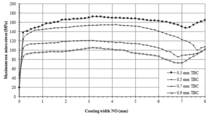
Fig.7 Normal stress variation as a function of coating thickness at bond coat
