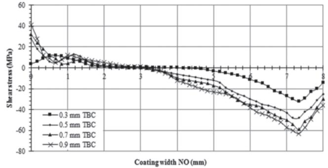
Fig.8 Shear stress variation as a function of coating thickness at bond coat surface
