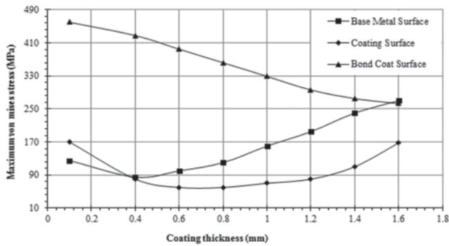
Fig.11 Maximum normal stress variation with coating thickness
