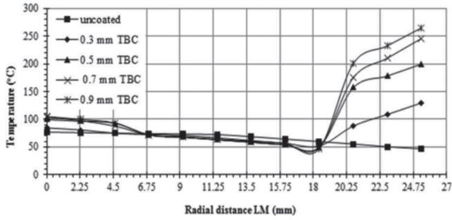
Fig.4(a) Top surface temperature distribution with coating thickness
