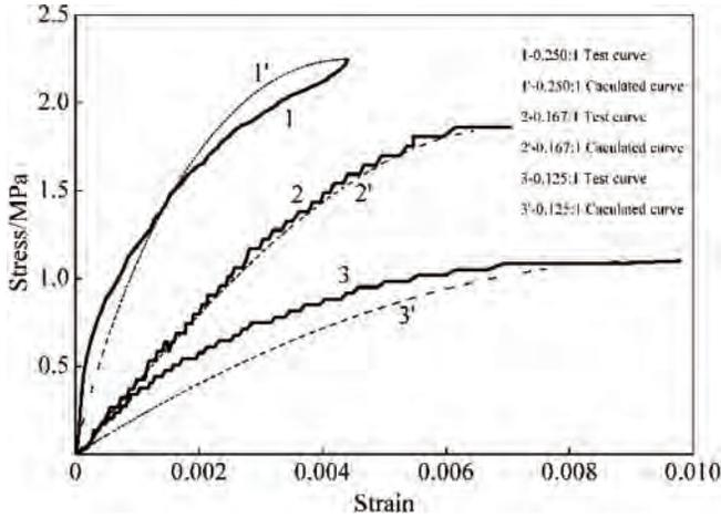
Fig.1 Stress-strain curves of backfill with different cement-tailing ratios
