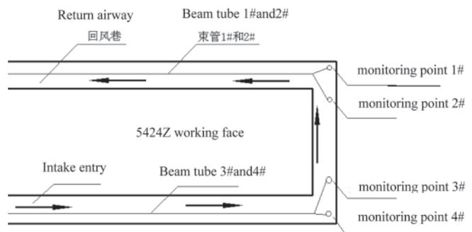
Fig.1 Schematic diagram of laying of beam tube monitoring points
