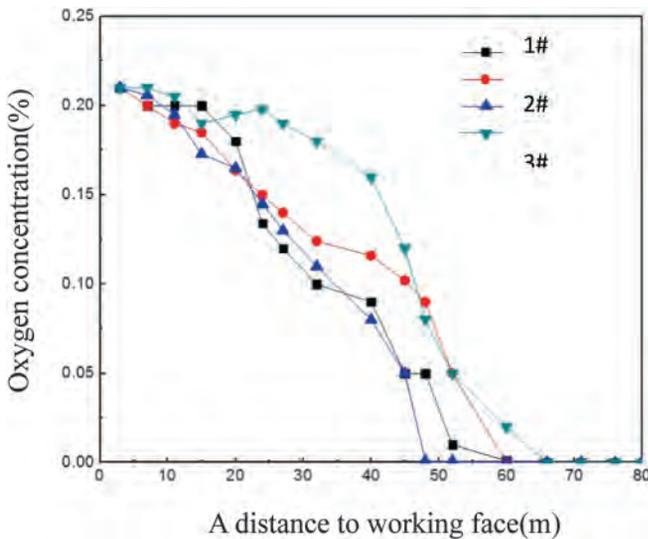
Fig.2 Line chart of measuring oxygen concentration distribution in gob
