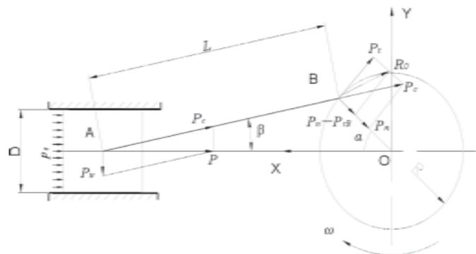
Fig.2 The connecting rod stress diagram
