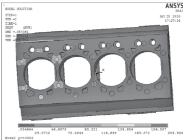
Fig.5 Stress distribution of the roof bolt hole at the 1st cylinder maximum explosion pressure condition
