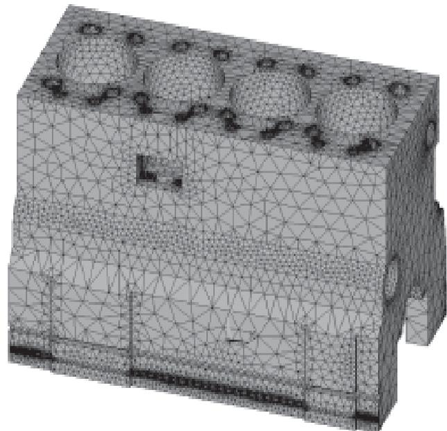
Fig.1 Diesel engine block's FEM
