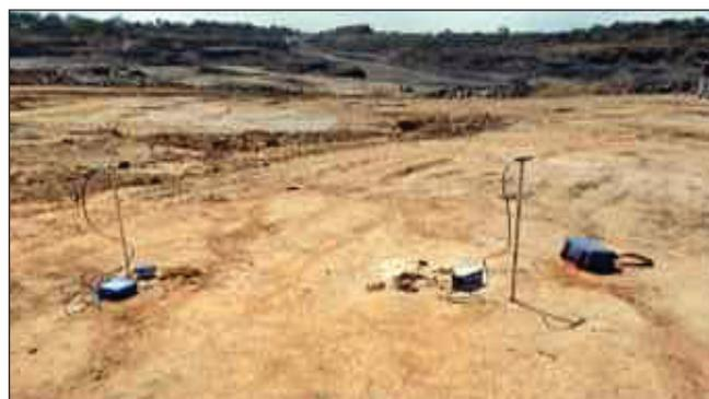
Fig.6: Seismographs monitoring the PPV at mine
