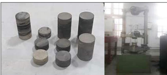
Fig.1: Rock samples for determining compressive and tensile strength of overburden rock
