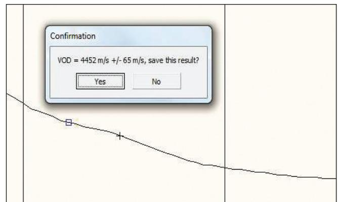
Fig.3: Analysis of in hole VOD
