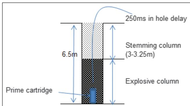
Fig.5: Blasthole section
