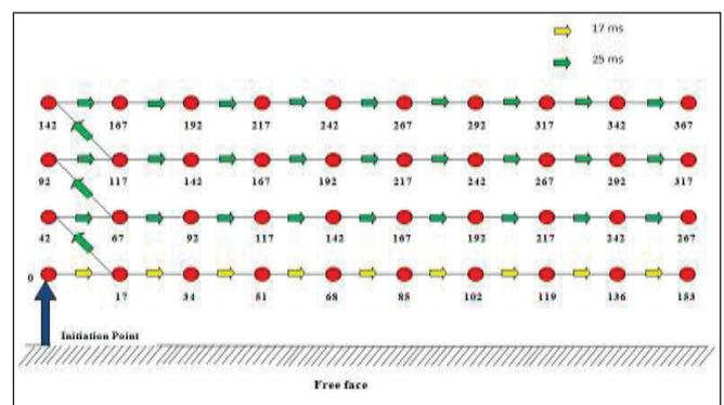
Fig.4: Drilling and firing pattern
