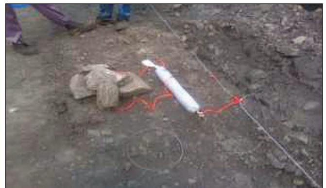
Fig.2: Deautriche set up for determination of unconfined VOD
